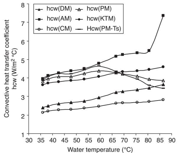
Fig. 2a. Variation of convective heat transfer coefficient ( $h_{cw}$ ) within temperature range of 35–85 °C.
