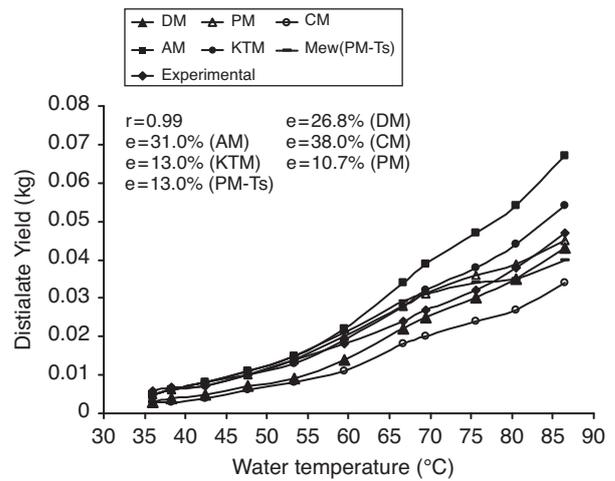
Fig. 3. Variation of distillate yield for different heat transfer models within temperature range of 35–85°C.
