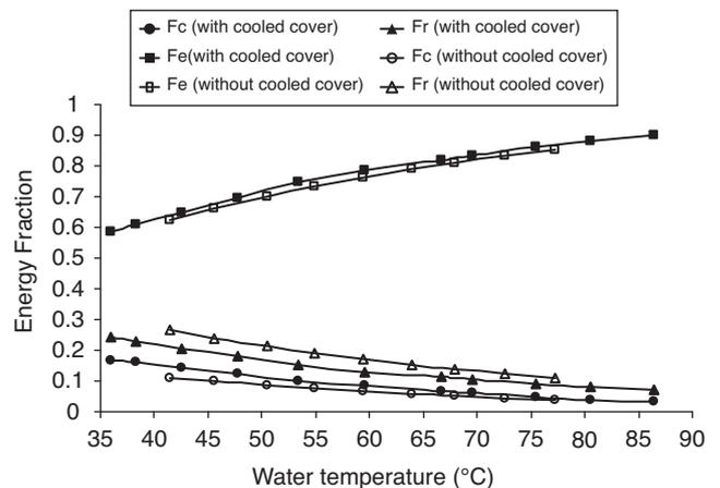
Fig. 4. Influence of energy fractions ( $F_r$ ,  $F_c$  and  $F_e$ ) within temperature range of 35–85°C for the cooled and without cooled condensing cover of solar still.
