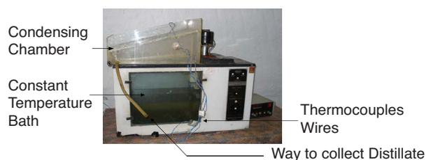
Fig. 1. Photograph of indoor distillation unit at 15° slope of the condensing cover.
