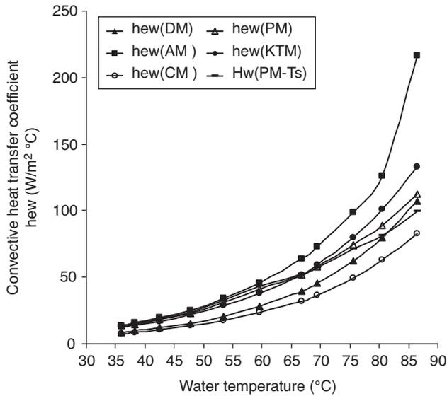
Fig. 2b. Variation of evaporative heat transfer coefficient ( $h_{ew}$ ) within temperature range of 35–85°C.
