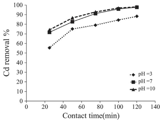
Fig. 2. Effect of pH on Cd adsorption using perlite,  $M = 10$  g and  $C_{Cd} = 2.6$  mg/l.
