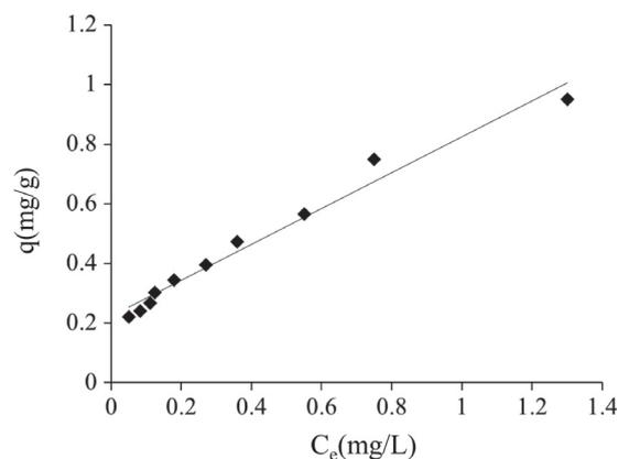
Fig. 5. Freundlich equation for Cd adsorption by perlite, pH = 7, T = 25 °C,  $C_e$ : Equilibrium metal concentration (mg/l).
