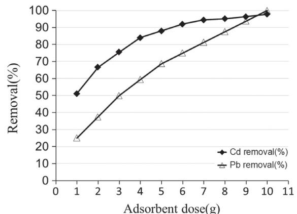
Fig. 4. Effect of different doses of adsorbent on Cd and Pb removal.
