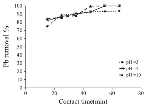
Fig. 1. Effect of pH on Pb adsorption using perlite,  $M = 10\text{ g}$ ,  $C_{\text{Pb}} = 11\text{ mg/l}$ .
