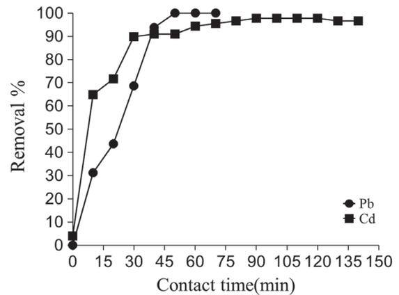
Fig. 3. Effect of contact time on Cd and Pb adsorption by 10 g perlite and at pH = 7.
