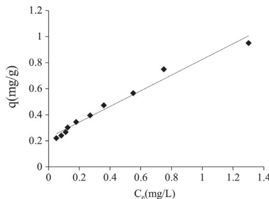
Fig. 6. Freundlich equation for Pb adsorption by perlite, pH = 7, T = 25 °C,  $C_e$ : Equilibrium metal concentration (mg/l).
