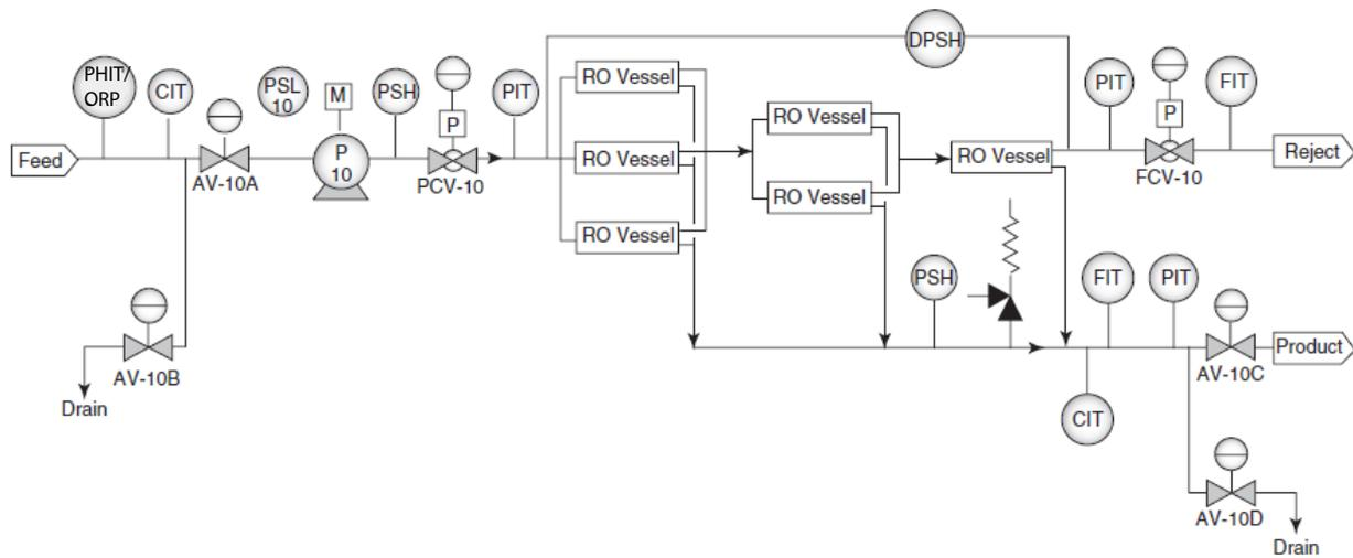
Fig. 3. A typical P&ID of a single-pass, three-stage RO/NF unit. PCV and FCV are automatic modulating pressure control and flow control valves, respectively. AV-x are automatic on/off valves.
