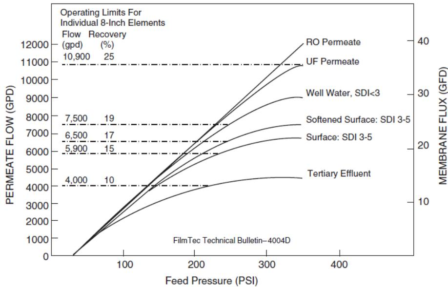
Fig. 1. Membrane flux characteristics of a thin-film composite polyamide membrane, spiral-wound RO module with various feed waters.
