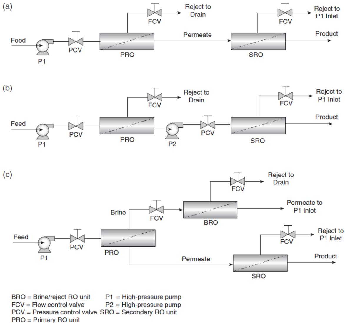
Fig. 4. RO system flow schematics: (a) two-pass RO without inter-pass pressure boosting; (b) two-pass RO with inter-pass pressure boosting; (c) two-pass RO with brine recovery.
