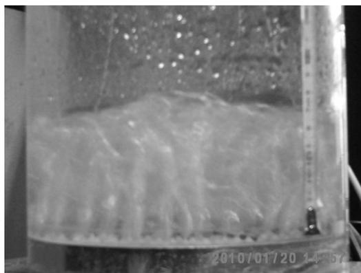
Fig. 5. Photo of bubbling in the humidifier.
