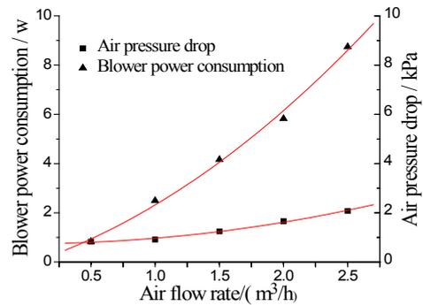
Fig. 6. Air pressure drop in humidifier and blower power consumption changed with air flow rate.
