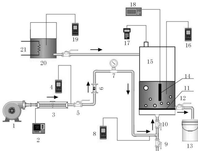
Fig. 2. Test-bed of bubbling humidification. 1 – blower; 2 – voltage transformer; 3 – air heater; 4, 8, 16, 19 – digital thermometer; 5, 9, 10, 12 – valve; 13 – water tank; 6 – flow meter; 7 – pressure gauge; 11 – sieve plate; 14 – heater; 15 – humidifier; 17 – hygrometer; 18 – temperature controller; 20 – hot water tank; 21 – water heater.
