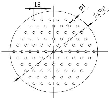
Fig. 3. Structure of a sieve plate.
