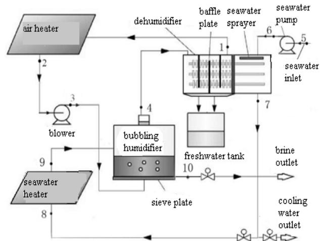
Fig. 1. Scheme of solar HD desalination with bubbling humidification.
