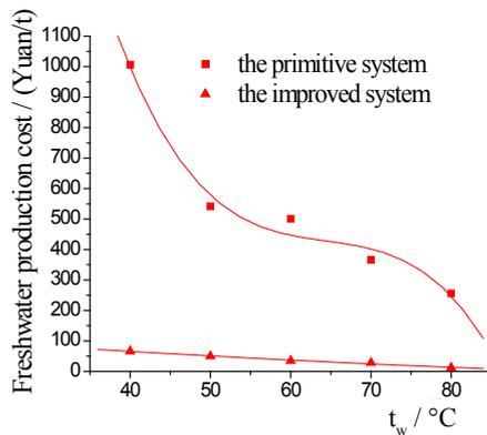
Fig. 11. Cost of fresh water production changed with temperature.
