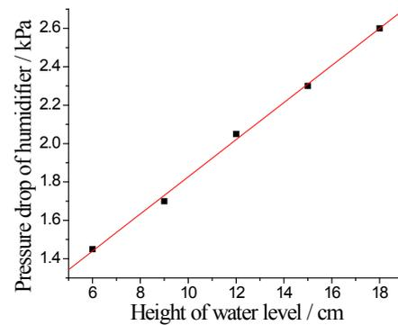
Fig. 7. Air pressure drop changed with the height of water level on sieve plate.
