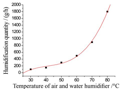
Fig. 8. Quantity of humidification changed with the temperature of air and water in the humidifier.
