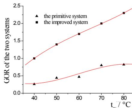
Fig. 10. GOR changed with the temperature of air and water in the humidifier.
