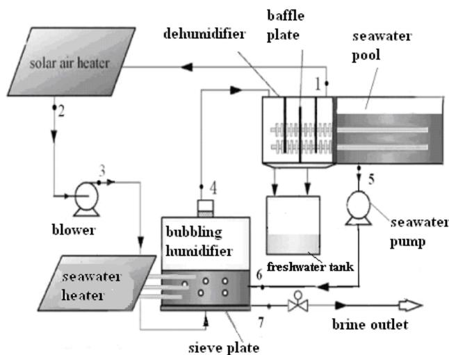
Fig. 9. Scheme of the improved solar HD desalination with bubbling humidifying.
