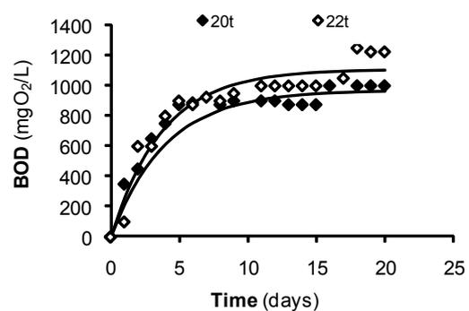
Fig. 2. Variation of the cork processing wastewater BOD with time. Samples collected after 20 and 22 tonnes of cork processed in the boiling stage.
