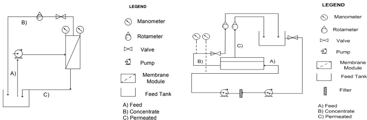
Fig. 1. Ultrafiltration (left) and nanofiltration (right) set-ups.
