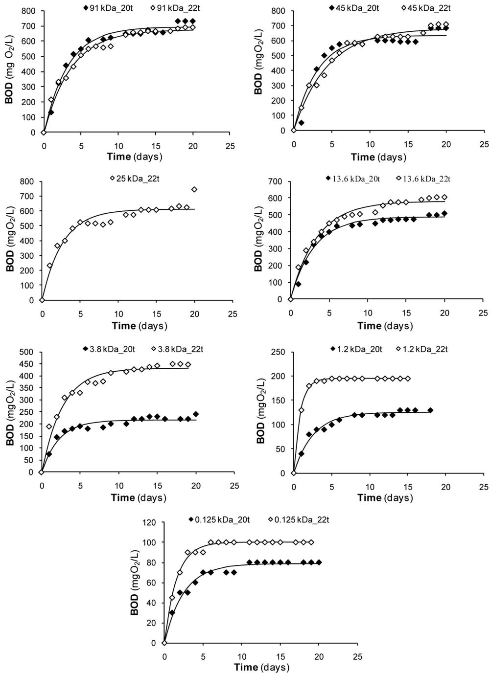
Fig. 3. Variation of permeates BOD with time for membranes with MWCO ranging from 0.125 kDa to 91 kDa.
