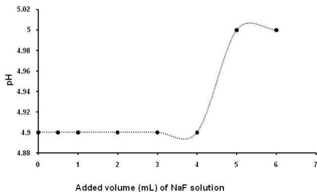
Fig. 6. The change in pH with the volume (mL) of NaF ( $5.2857 \times 10^{-3}$  M) solution added to system 8.
