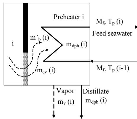
Fig. 3. Flow diagram of a typical pre-heater.
