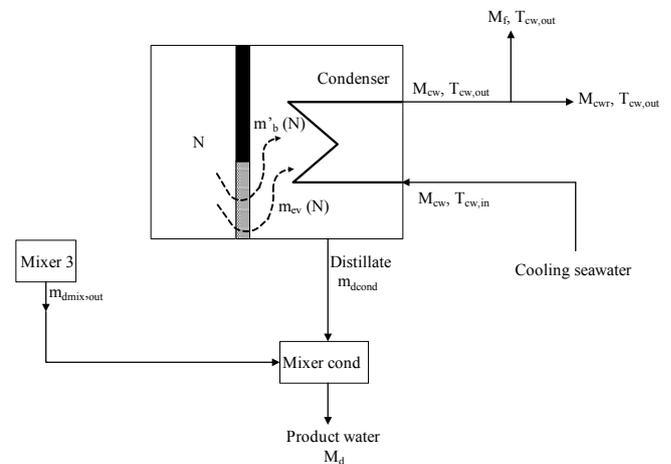
Fig. 8. Flow diagram of the end condenser.
