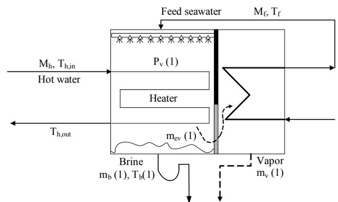
Fig. 2. Flow diagram of the heater (effect 1).
