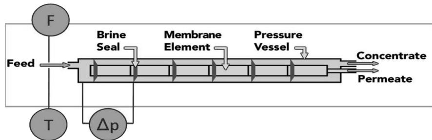
Fig. 1. Principle of the in-line biofouling monitor.
