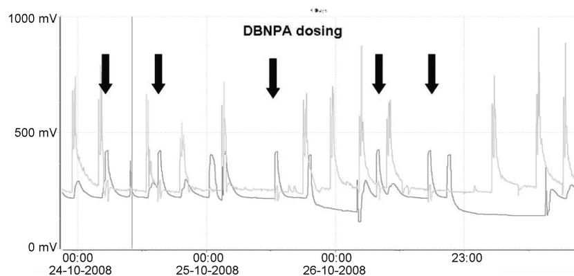
Fig. 8. ORP potential concentrate of RO-3 with intermittent DBNPA dosing (dark gray) and after neutralization with sodium bisulphite (light gray).
