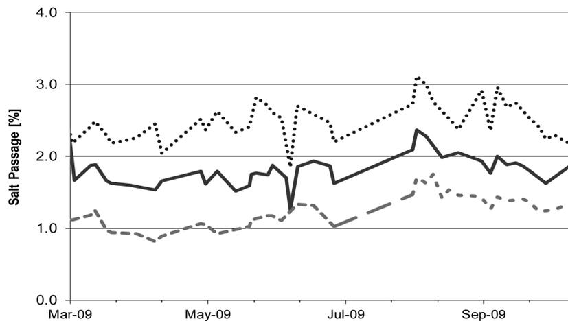
Fig. 7. Normalized salt passage (based on conductivity); RO-1 (black), RO-2 (dotted black) and RO-3 (striped gray).
