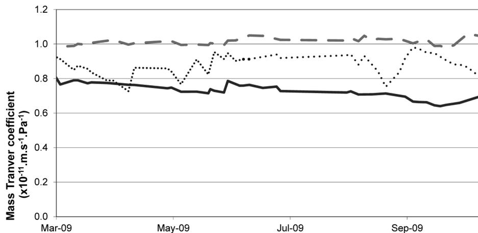
Fig. 6. Mass transfer coefficient: RO-1 (black), RO-2 (reference; dotted black) and RO-3 (striped gray).
