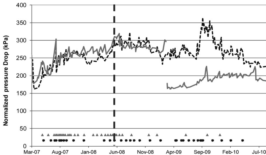
Fig. 5. Normalized pressure drop in RO-3 with DBNPA (gray) and RO-2 as reference, without any biocide (dotted black). At the bottom, triangles and circles indicate CIP of both RO units.
