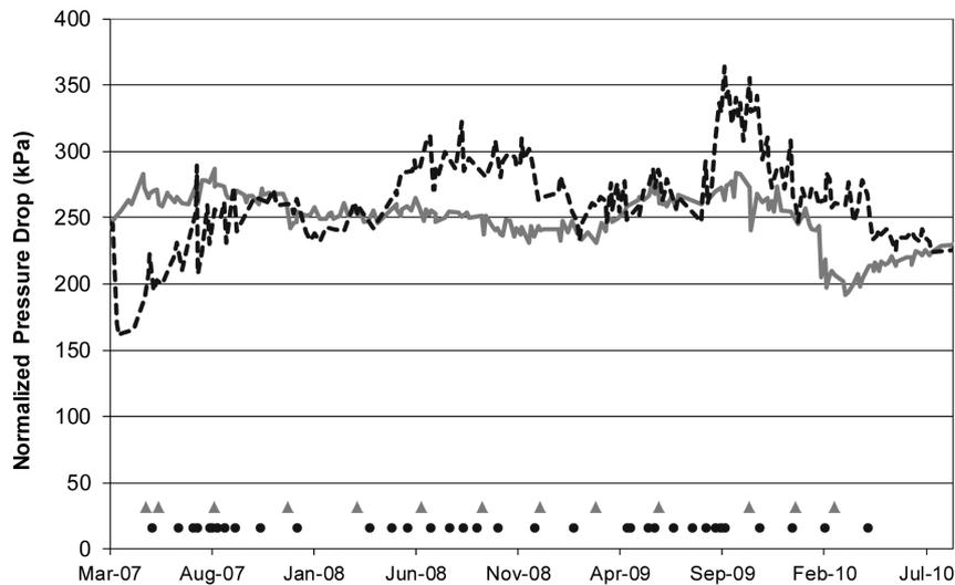
Fig. 4. Normalized pressure drop RO-1 with dosing PAA (gray) and RO-2 (dotted black) without any biocide (reference). At the bottom, triangles and circles indicate CIP of both RO units.
