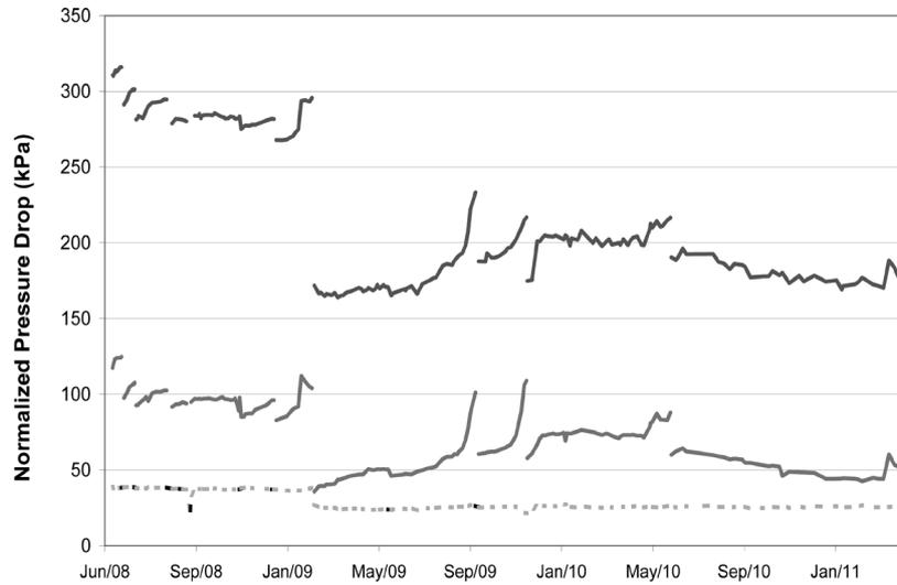
Fig. 3. Normalized pressure in RO-3 across first stage (black), first element (thick striped gray) and average last 5 elements (dotted light gray).
