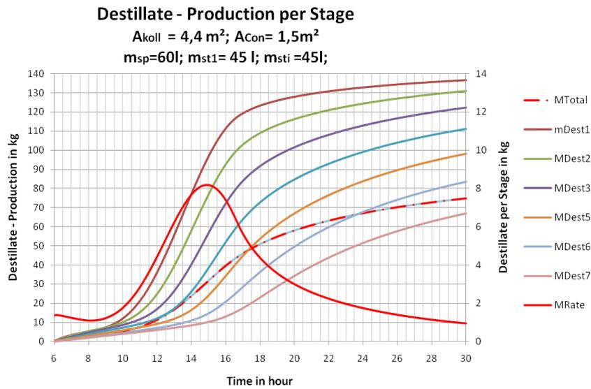
Fig. 8. Simulation results for Akutsima, Namibia – production rate profiles for the stages of the desalination tower.
