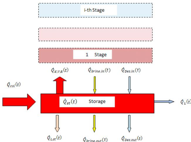
Fig. 5. Schematic drawing of the flow rates in the storage tank of the desalination system.
