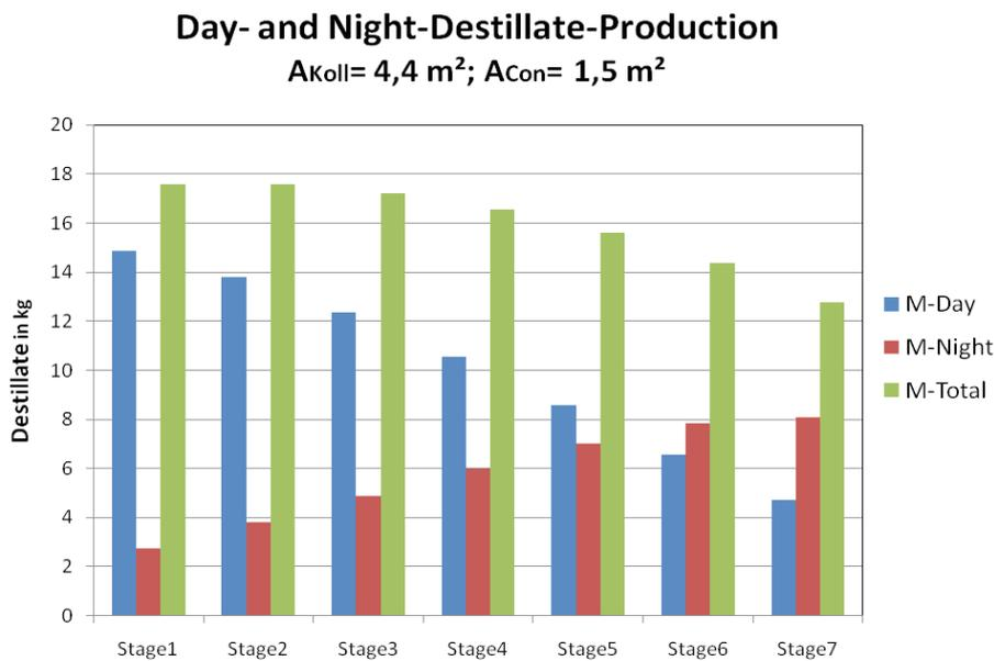
Fig. 9. Simulation results for Akutsima, Namibia – production rate profiles for the stages in column form.
