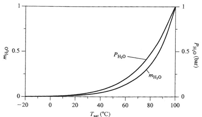
Fig. 1. Vapor pressure of water and mass concentration of water in saturated air at  $P = 1.013$  bar. Adapted from [10].
