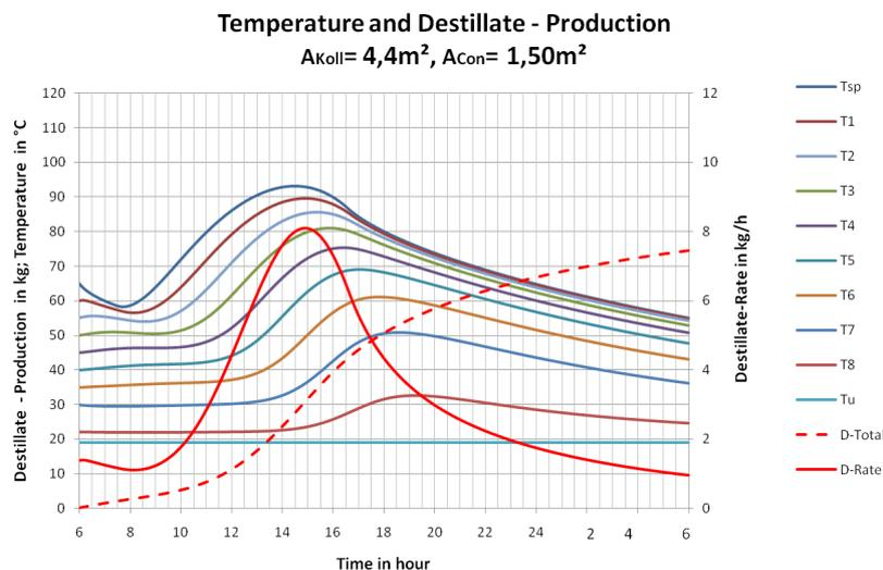
Fig. 7. Simulation results for Akutsima, Namibia – temperature profile, tower rate, and cumulative tower rate profiles.
