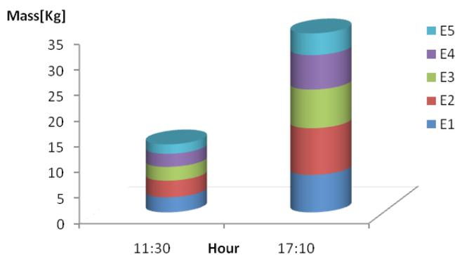
Fig. 6. Desalinated water production (for a 24-h period) at the hour of collections: 11:30 and 17:10 h. E1–E5 represent stage 1–stage 5.
