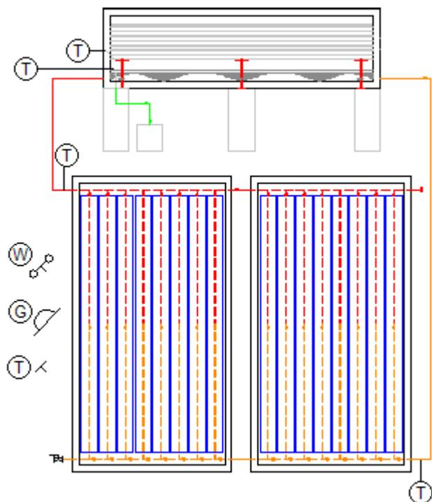
Fig. 4. Schematic drawing of the desalination system with indication of the measurement points: T – thermocouple, W – anemometer, G – pyranometer.
