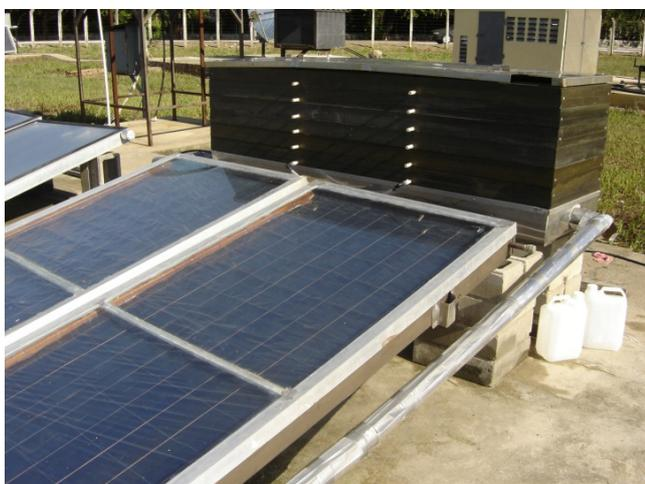
Fig. 3. System manufactured in Brazil with 6 stages and flat plate solar collectors.
