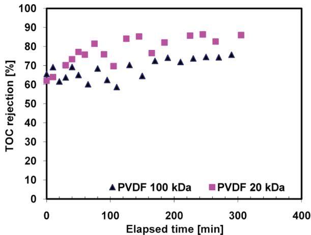
Fig. 13. TOC rejection as a function of time with high and low MWCO membranes.
