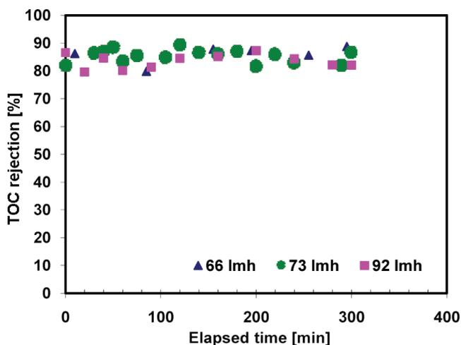
Fig. 20. Effect of the initial permeate flux on the TOC rejection (set III).
