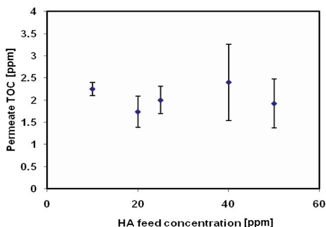
Fig. 21. Mean permeate TOC vs. HA feed concentration (PVDF 100 kDa membrane).
