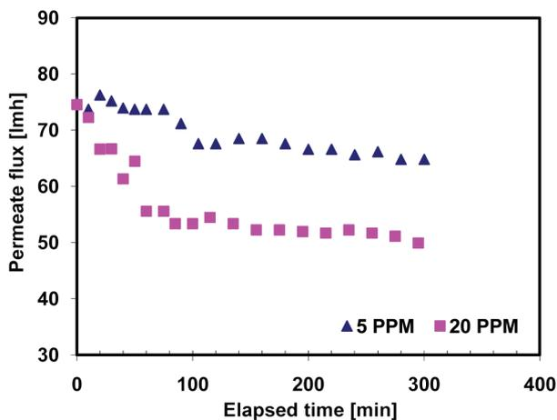
Fig. 16. Effect of HA feed solution concentration on the flux decline with time.
