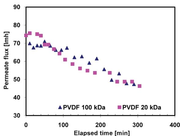
Fig. 12. Permeate flux as a function of time with high and low MWCO membranes.
