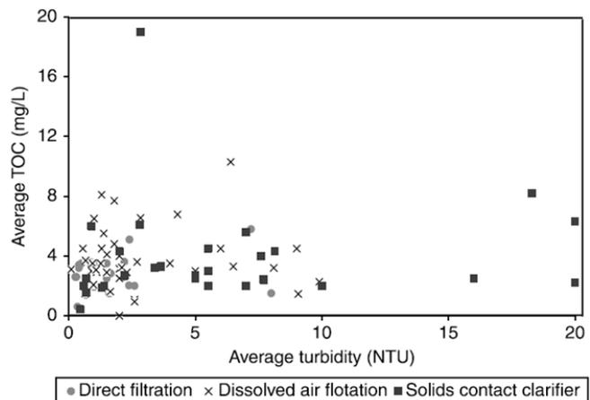
Fig. 3. Average levels of TOC and turbidity measured in different treatment plants [5].
