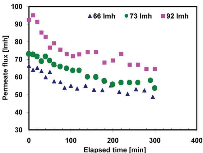
Fig. 18. Effect of the initial permeate flux on the permeate flux decline with time (set III).
