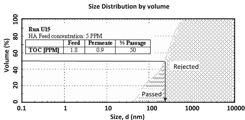
Fig. 5. Illustration of the “cut” evaluation method for a UF test (run U15).
