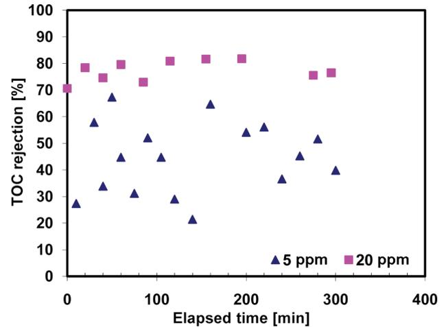
Fig. 17. Effect of HA feed solution concentration on the TOC rejection.
