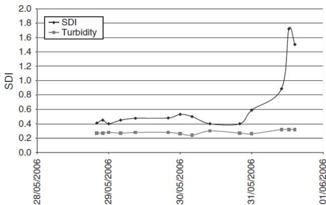
Fig. 2. SDI and turbidity measurements of pretreated feed water [3].
