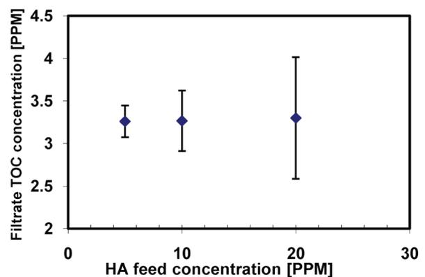
Fig. 7. Mean filtrate TOC content vs. HA feed concentration in filtrations performed in a fresh bed or in a cleaned bed.
