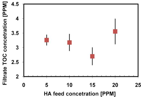
Fig. 8. Mean filtrate TOC content vs. HA feed concentration in filtrations performed in either a cleaned bed or a used bed.
