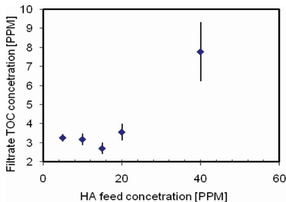
Fig. 9. Mean filtrate TOC content at all HA feed concentrations in all runs.
