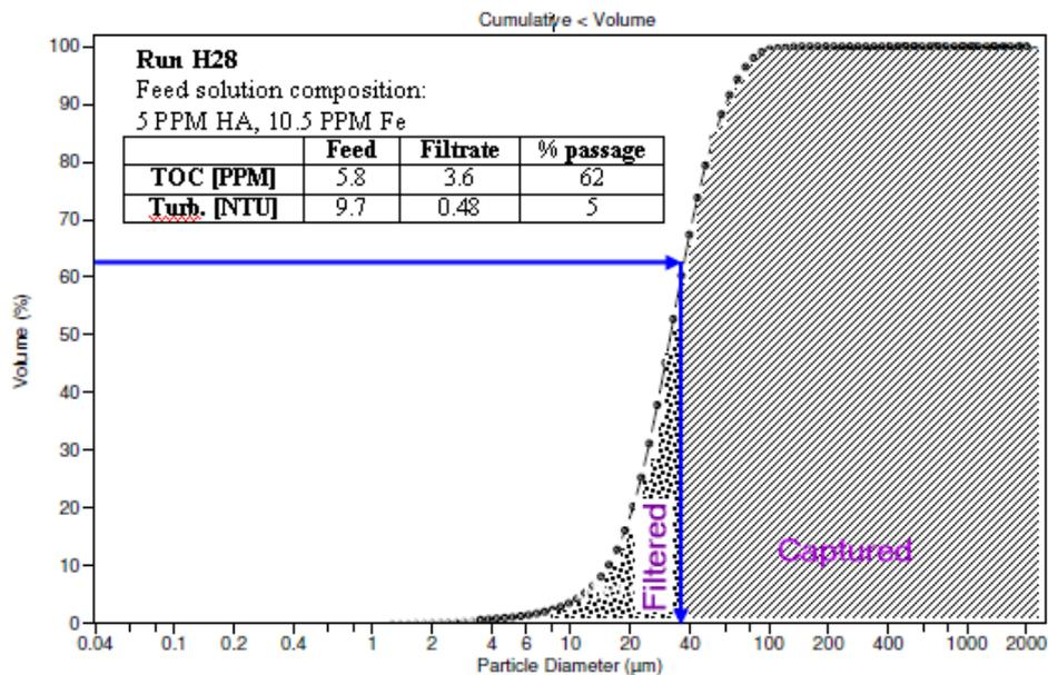
Fig. 4. Illustration of the “cut” evaluation method for a sand filtration test (run H28).
