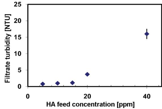
Fig. 10. Mean filtrate turbidity vs. HA feed concentration in all runs.
