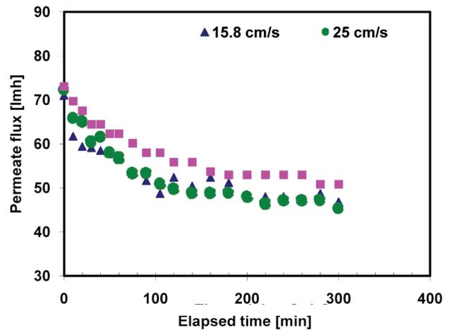
Fig. 14. Effect of flow velocity on permeate flux.
