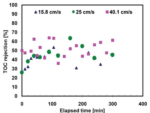
Fig. 15. Effect of flow velocity on TOC rejection.
