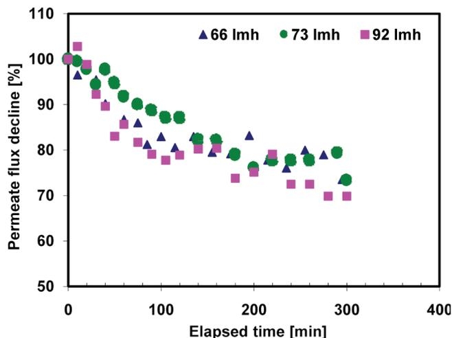
Fig. 19. Effect of the initial permeate flux on the fractional flux decline with time (set III).
