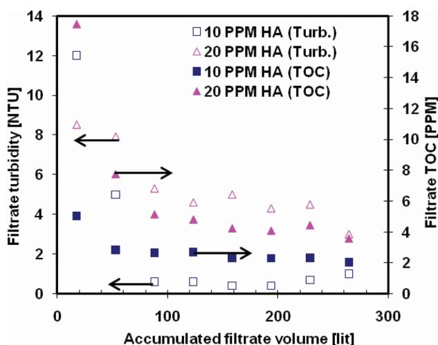
Fig. 6. Filtrate turbidity and TOC content as a function of total filtrate volume at two HA feed concentrations.
