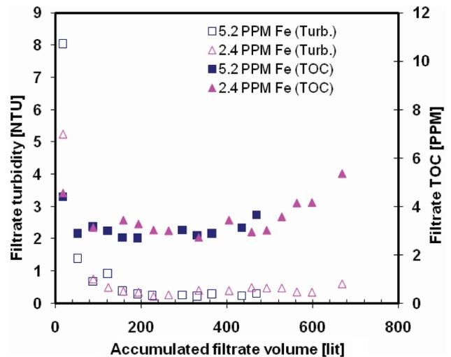
Fig. 11. Filtrate turbidity and TOC content vs. accumulated filtrate volume at two different Fe feed concentrations (set I runs).
