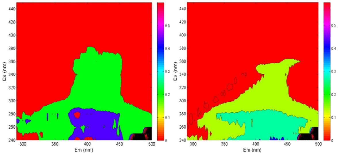
Fig. 8. FEEM, Moni, Apr-2009 (raw water left, UF permeate right).
