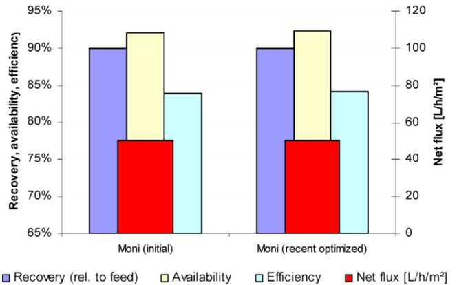
Fig. 5. Graph showing Moni UF system recovery, availability, efficiency and net flux.
