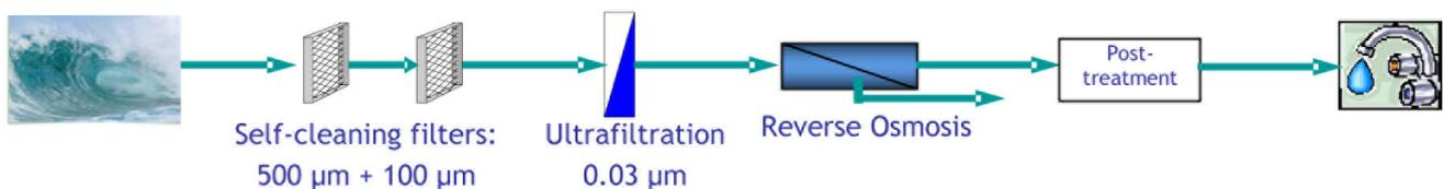
Fig. 1. Simple desalination process diagram used at Moni desalination plant.
