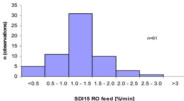
Fig. 6. Standard SDI measurements in the RO feed stream.
