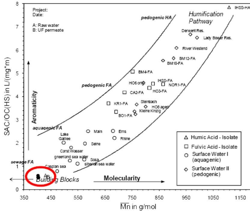
Fig. 7. Humic substances concentration vs. molecular weight (figure facilitated by UNESCO IHE).
