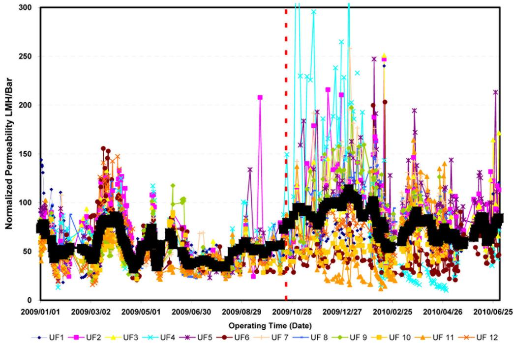
Fig. 4. Normalized permeability evolution for all individual UF racks and system average.
