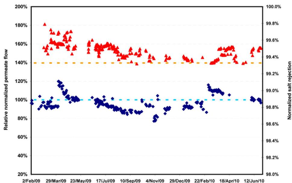
Fig. 9. Relative normalized permeate flow (blue diamonds) and normalized salt rejection (red triangles) of the RO system.
