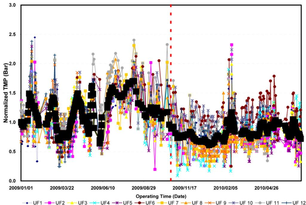
Fig. 3. Normalized TMP evolution for all individual UF racks and system average.
