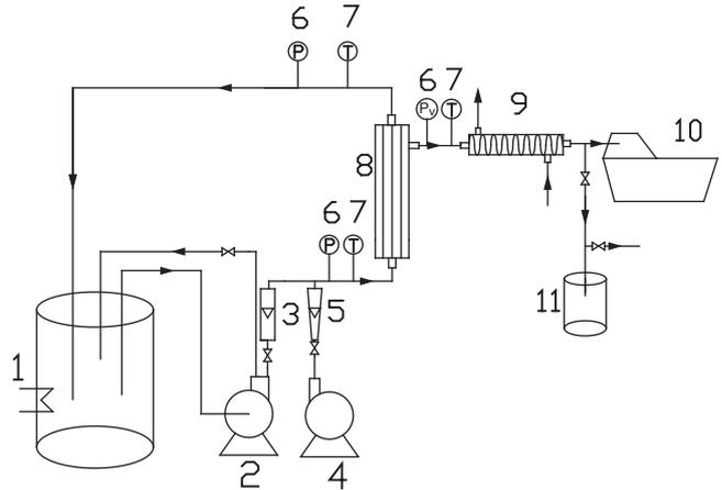
1. water bath; 2. pump; 3. liquid flowmeter; 4. gas pump; 5. gas flowmeter; 6. manometer; 7. thermometer; 8. hollow fiber membrane module; 9. condenser; 10. vacuum pump; 11. product collection
