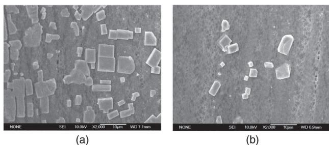
Fig. 5. SEM photograph of membranes used in VMD (a) and AVMD (b) process.
