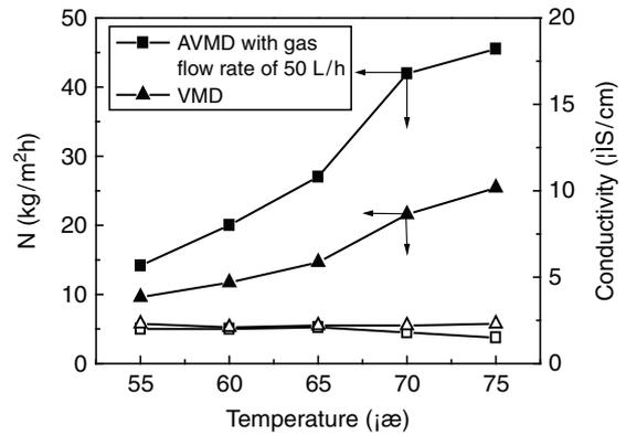
Fig. 3. Effect of feed temperature on the performance of VMD and AVMD processes.
