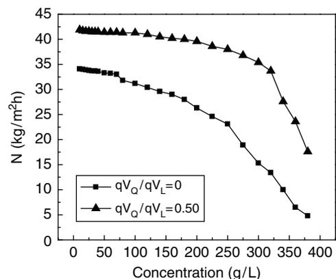
Fig. 4. Effect of feed NaCl concentration on the performance of AVMD process.
