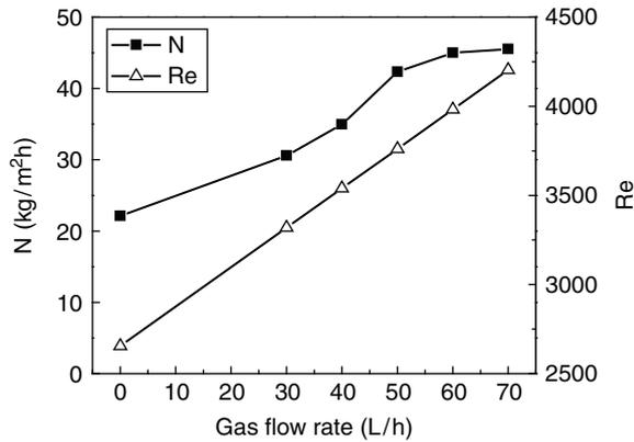
Fig. 2. Effect of feed gas flow rate on the performance of AVMD process.
