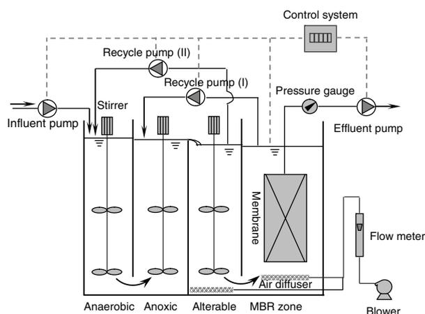
Fig. 1. Flow diagram of the MBR setup.
