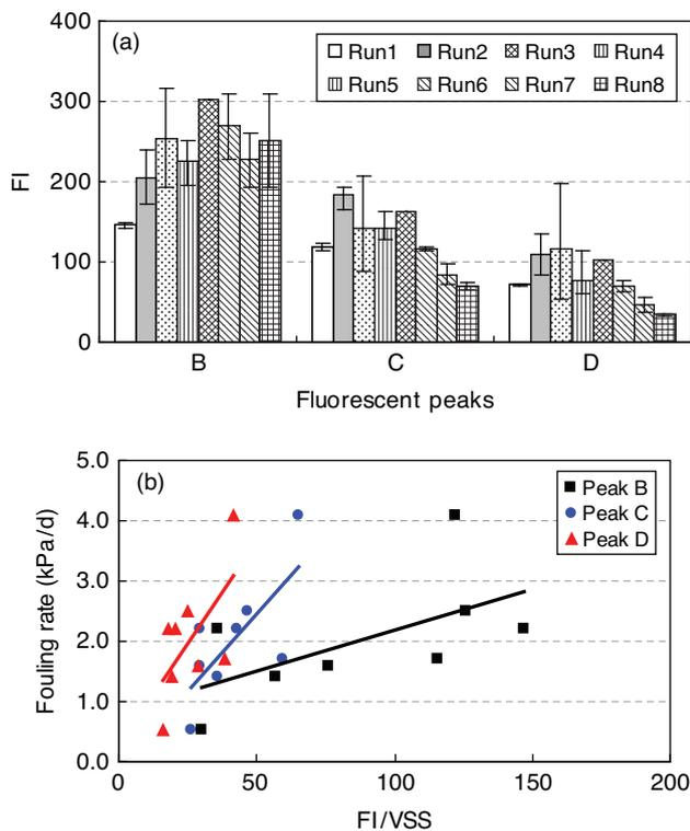
Fig. 6. (a) FI of Peaks B, C and D in the 8 runs; (b) correlations of FI/VSS with membrane fouling rate.
