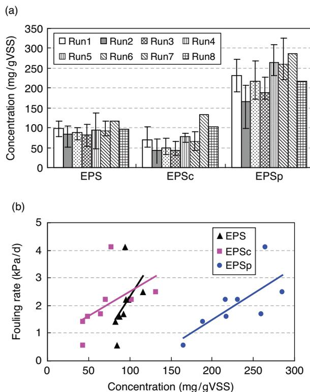
Fig. 4. (a) Variations of EPS,  $EPS_c$  and  $EPS_p$  in 8 runs; (b) correlations of EPS,  $EPS_c$  and  $EPS_p$  with membrane fouling rate.
