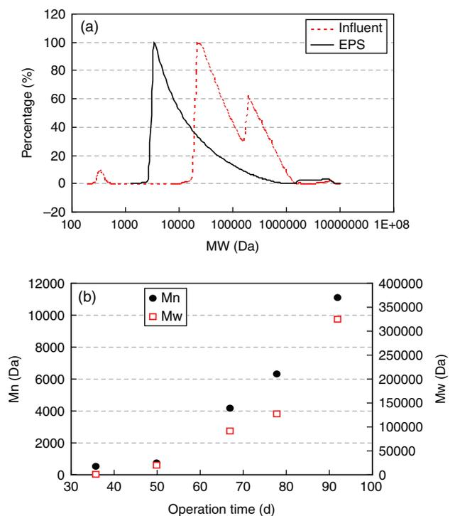
Fig. 7. (a) MW distribution of EPS and influent wastewater; (b) variations of  $M_n$  and  $M_w$  during the operation in Run 2.
