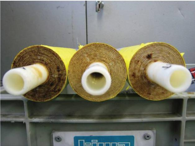
Fig. 4. Visual inspection of the three membrane elements at the inlet side.
