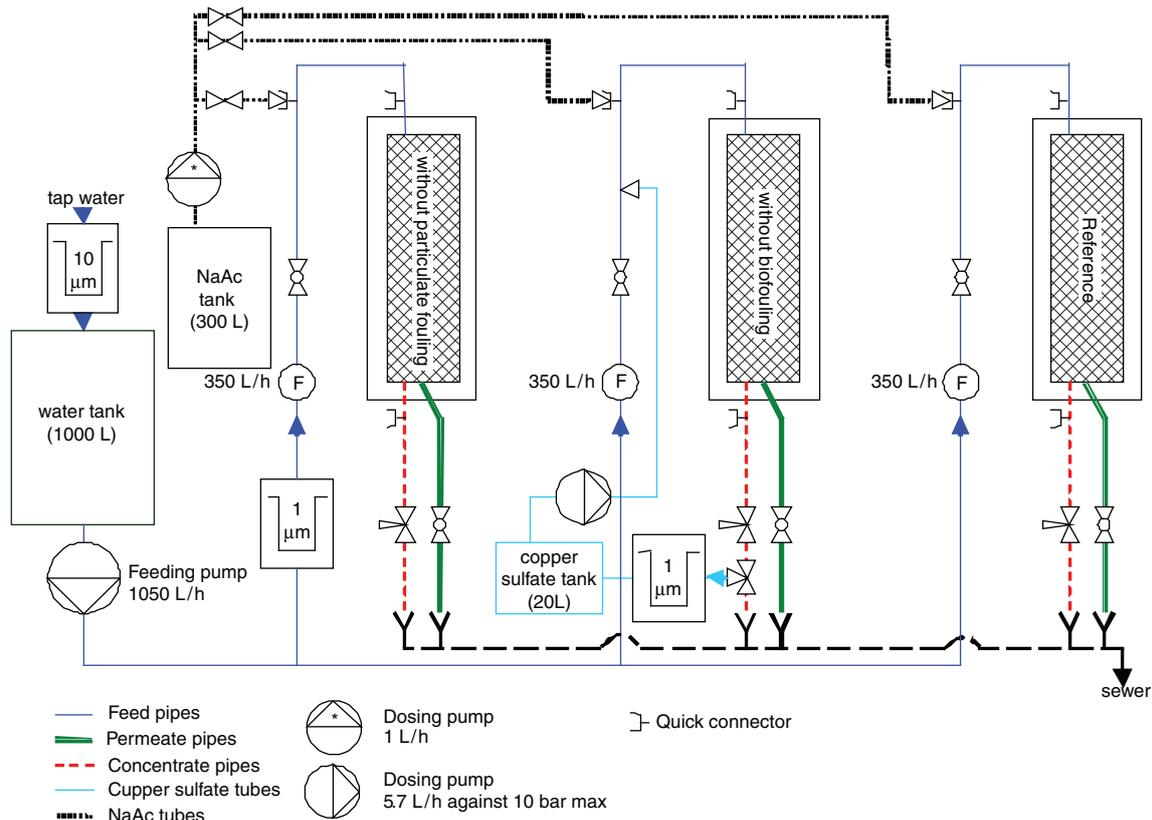
Fig. 2. Schematic depiction of the three element set-up used for the study of the influence of particles on biofouling.
