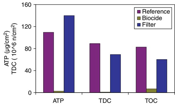
Fig. 6. Biological and organic deposits determined after membrane autopsy.
