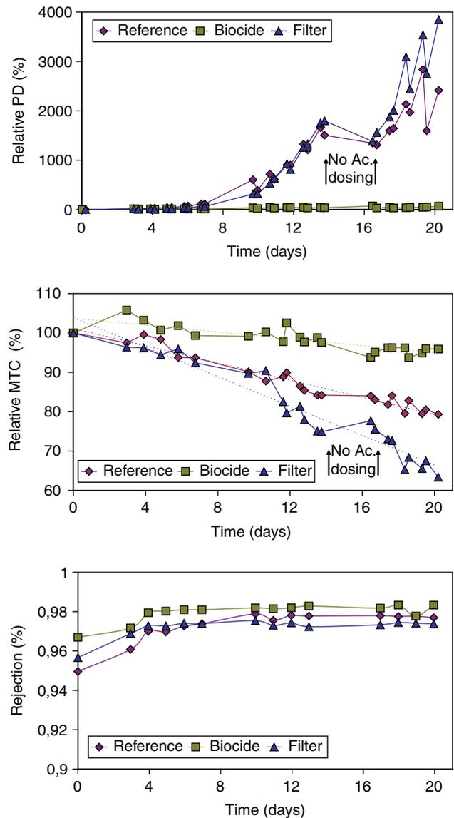
Fig. 3. Relative membrane transfer coefficient (MTC), relative pressure drop (PD) and rejection in function of time.
