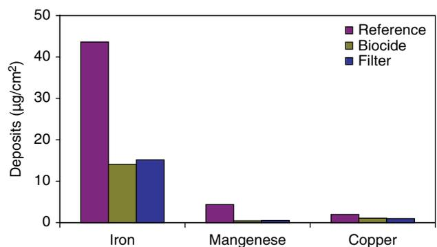
Fig. 7. Inorganic deposits determined after membrane autopsy.
