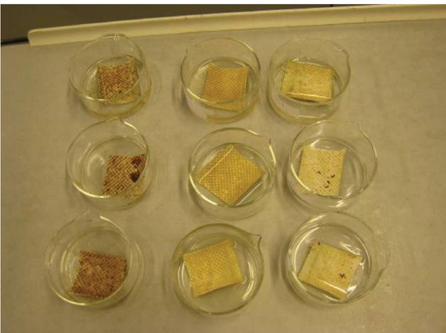
Fig. 5. Membrane coupons obtained from the three elements (left to right) at different positions of the membrane leaf from top to bottom.
