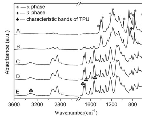
Fig. 2. FTIR spectra of PVDF/TPU blends with various mass ratios (A) 100/0, (B) 75/25, (C) 50/50, (D) 25/75, (E) 0/100.
