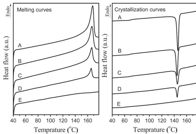
Fig. 4. DSC melting and crystallization behavior of PVDF/TPU blends with various mass ratios: (A) 100/0, (B) 75/25, (C) 50/50, (D) 25/75, (E) 0/100.
