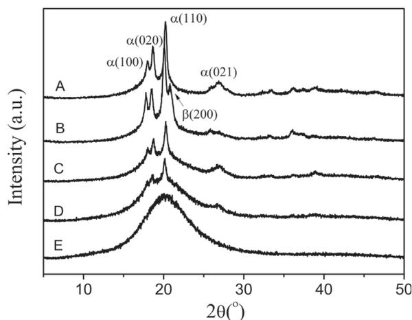
Fig. 3. WAXD diffractograms of PVDF/TPU blends with various mass ratios: (A) 100/0, (B) 75/25, (C) 50/50, (D) 25/75, (E) 0/100.
