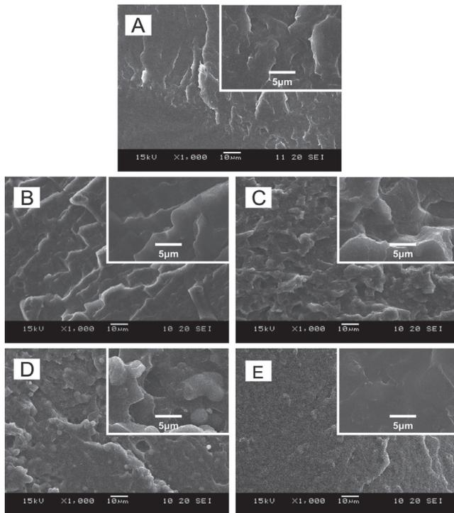
Fig. 1. SEM micrographs of cross section of PVDF/TPU blends with various mass ratios (A) 100/0, (B) 75/25, (C) 50/50, (D) 25/75, (E) 0/100.
