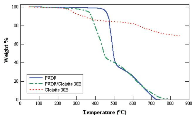
Fig. 6. TGA thermograms of Cloisite® 30B, original PVDF and PVDF/nanoclay membranes.
