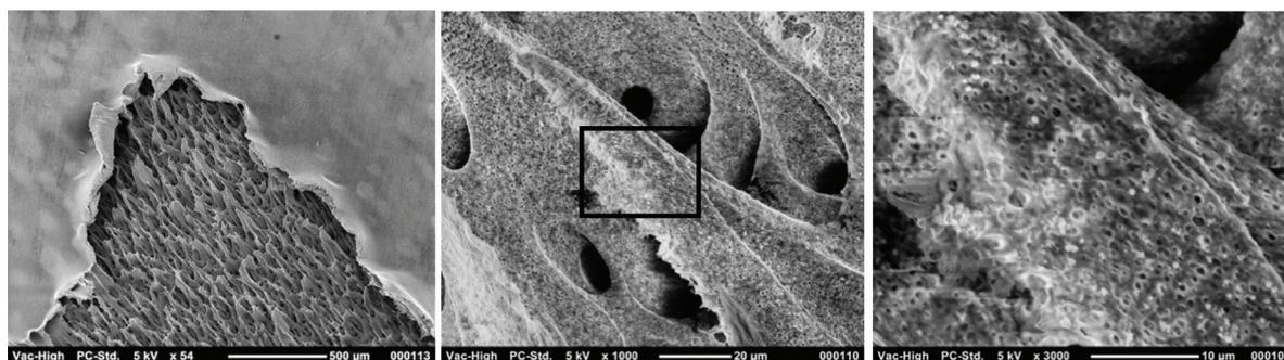
Fig. 5. SEM micrographs of the inner core of a PVDF/Cloisite® 30B membrane with increasing magnification (left to right).
