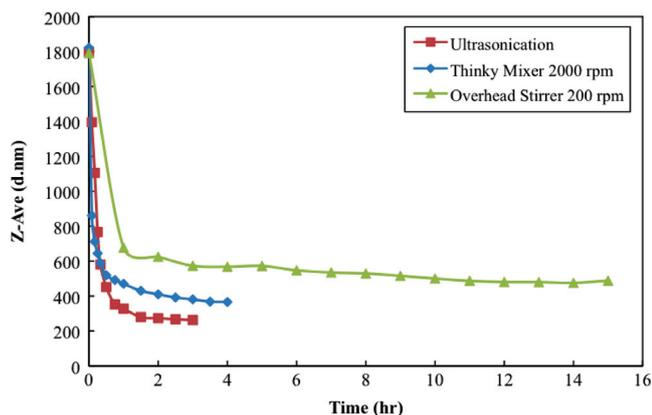
Fig. 2. Z-average particle size of Cloisite® 30B dispersed in NMP vs mixing time.
