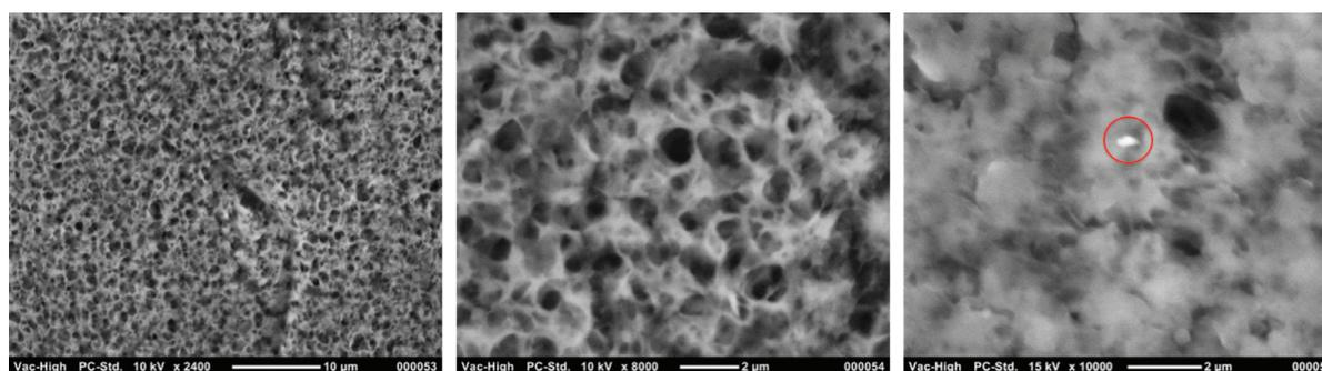
Fig. 4. SEM micrographs of the top surface of a PVDF/Cloisite® 30B membrane with increasing magnification (left to right). Right image is close-up of the 'dense' region observed in the middle image.
