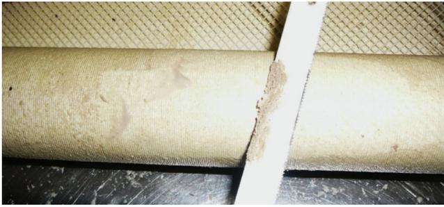
Fig. 2. Scale scraped from the NF membrane.
