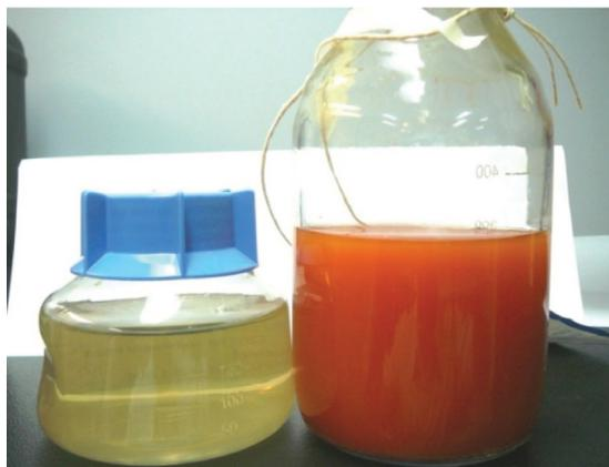
Fig. 1. TSF water before and after air sparging.
