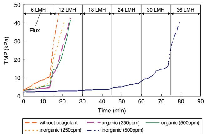
Fig. 3. Flux-TMP profile with the coagulant concentration.
