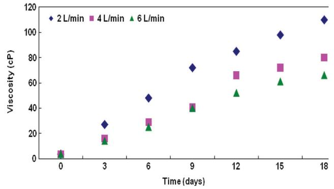
Fig. 8. Viscosity profile at various aeration rates.
