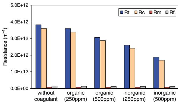
Fig. 4. Variation of resistances at different coagulant concentrations.
