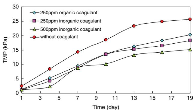
Fig. 10. TMP increase at different coagulation conditions.
