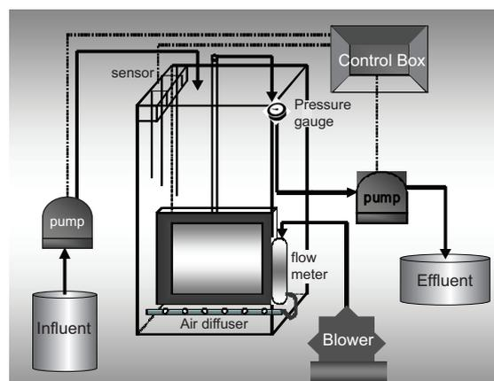
Fig. 1. Schematic diagram of the ADMF system.
