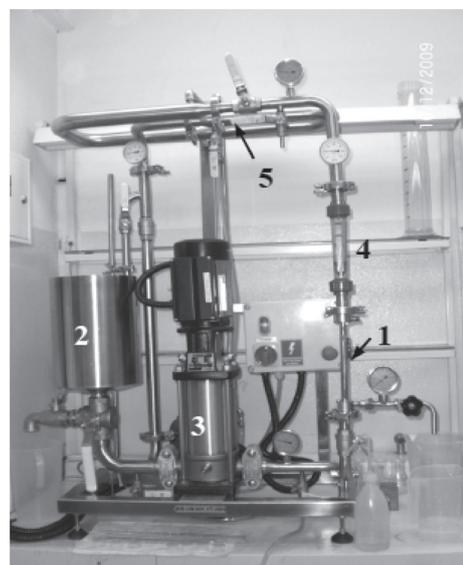
Fig. 1. Laboratory UF installation J.A.M INOX PRODUKT. 1 – ceramic module, 2 – feed tank, 3 – Grundfos pump, 4 – rotameter, 5 – thermostat.
