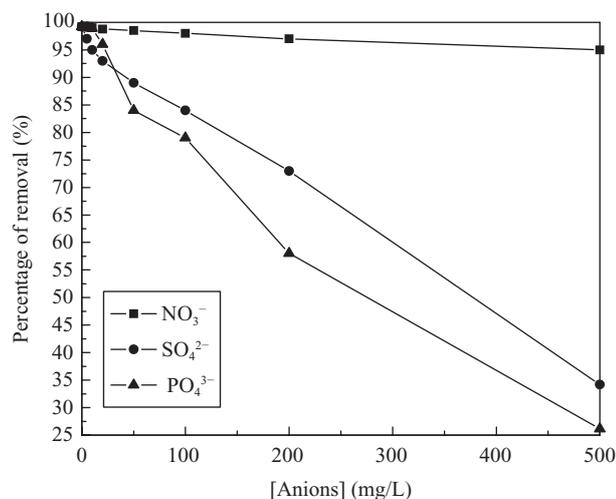
Fig. 5. Effect of other anions on the chloride removal.
