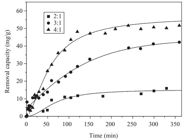
Fig. 3. Effect of Mg/Al molar ratio of CLDH on the chloride removal.
