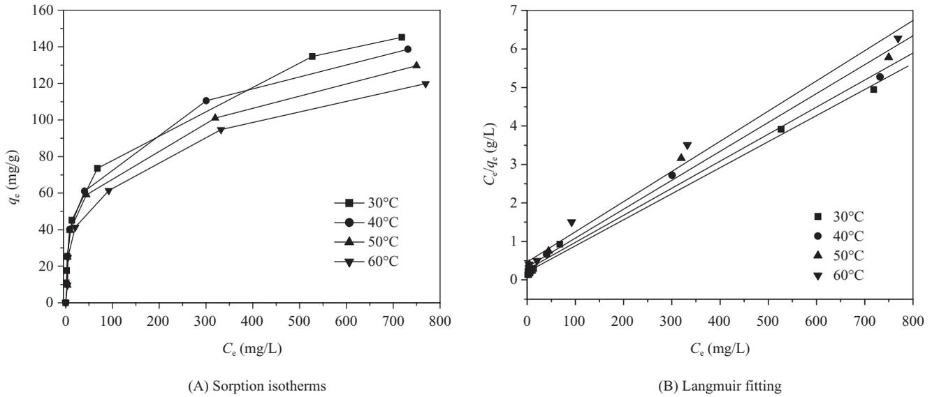
Fig. 1. The sorption isotherms of chloride removal by CLDH.
