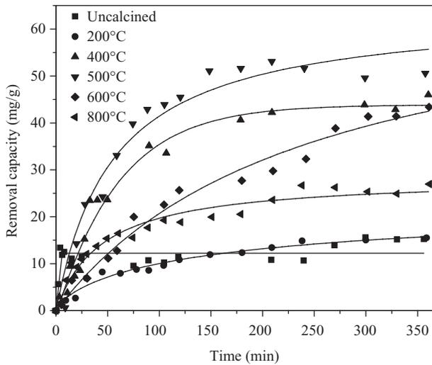
Fig. 2. Effect of calcinations temperature of CLDH on the chloride removal.
