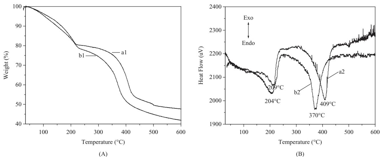
Fig. 7. TG and DTA profiles for (a) MgAl-CO<sub>3</sub> LDHs and (b) CLDH after chloride removal.
