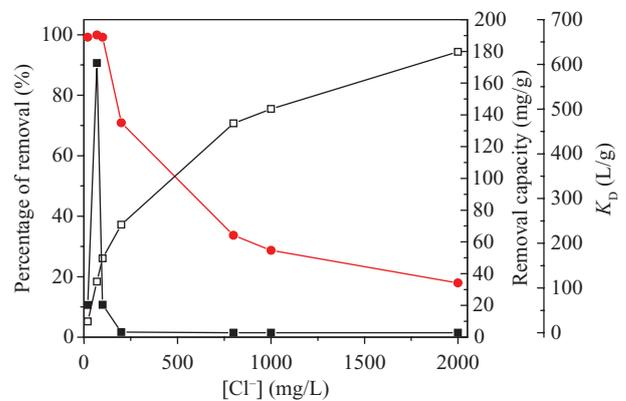
Fig. 4. Effect of initial chloride concentration on the chloride removal. (□) removal capacity vs. initial chloride concentration; (●) percentage of removal vs. initial chloride concentration; (■) distribution coefficient  $K_D$  vs. initial chloride concentration.
