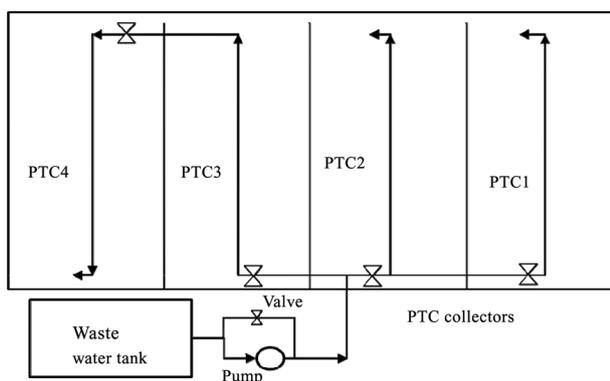
Fig. 1. Layout of the installed solar water disinfecting systems.
