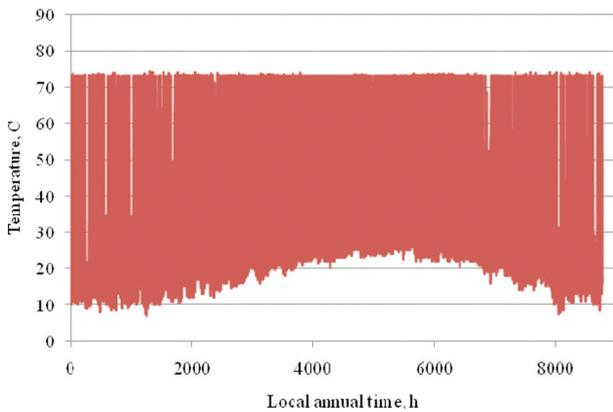
Fig. 10. Hourly variation of the collector outlet temperature of PTC2.
