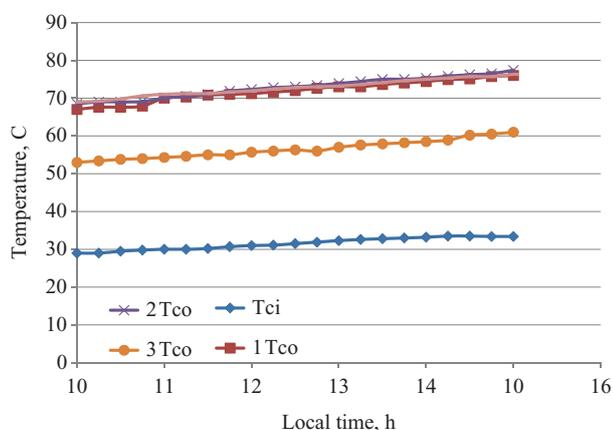
Fig. 4. Inlet and outlet temperatures variation of the concentrators on 5/7/2007.
