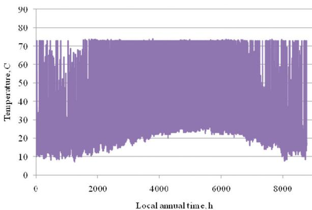
Fig. 11. Hourly variation of the collector outlet temperature of PTC4.
