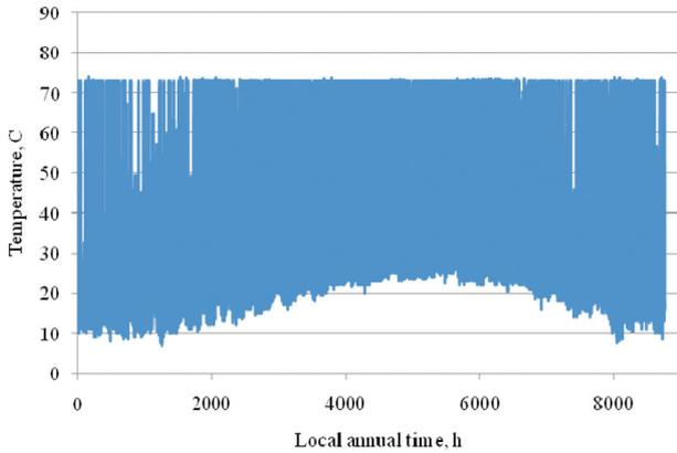
Fig. 9. Hourly variation of the collector outlet temperature of PTC1.
