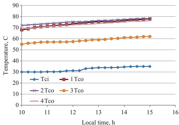
Fig. 3. Temperatures variation of the inlet and outlet flow on 4/7/2007.
