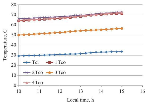
Fig. 5. Inlet and outlet temperatures variation of the concentrators on 7/7/2007.
