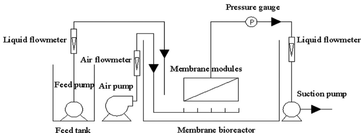
Fig. 1. Schematic diagram of membrane bioreactor.
