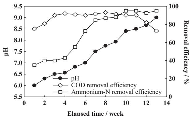
Fig. 4. COD and ammonium-N removal with different pH value.
