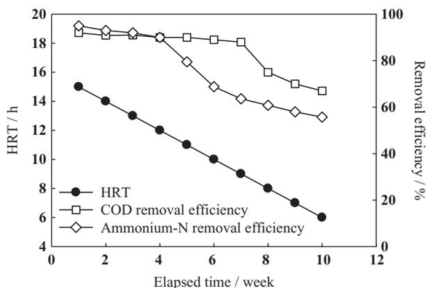
Fig. 6. COD and ammonium-N removal with different HRT.
