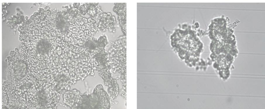
Fig. 5. Micrographs of sludge structure in wastewater without seawater (left) and with 50% seawater (right).
