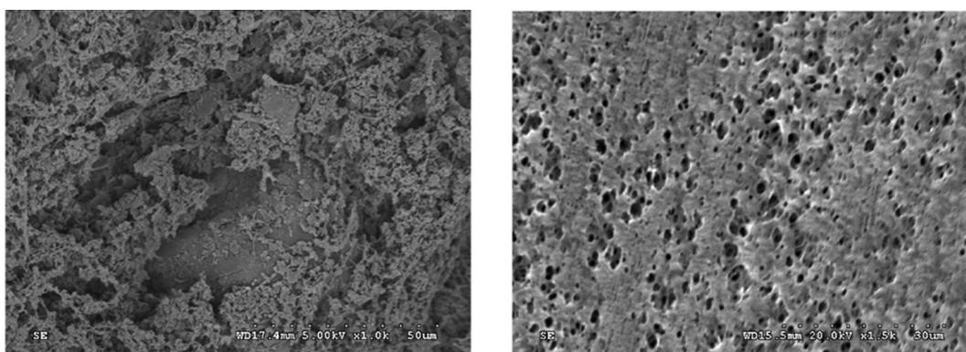
Fig. 8. SEM images of membrane surface before (left) and after (right) membrane cleaning.
