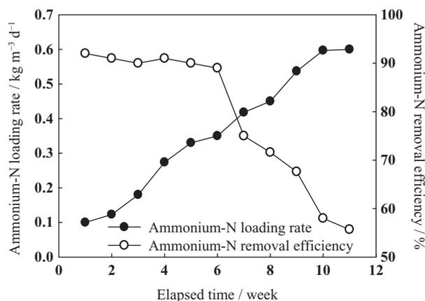
Fig. 3. Ammonium-N removal efficiency with different ammonium-N loading rates.
