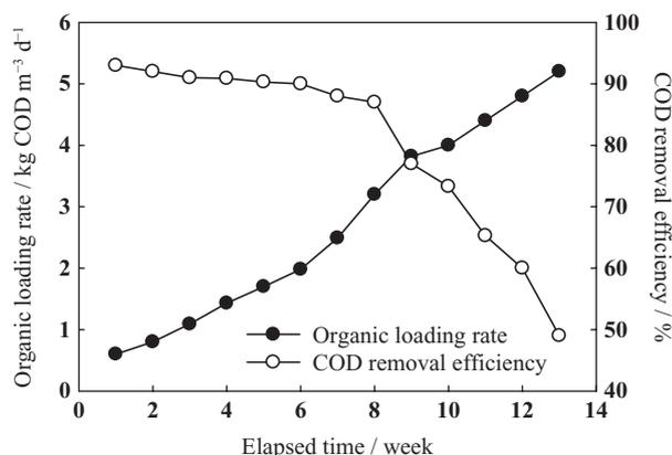
Fig. 2. COD removal efficiency with different organic loading rates.
