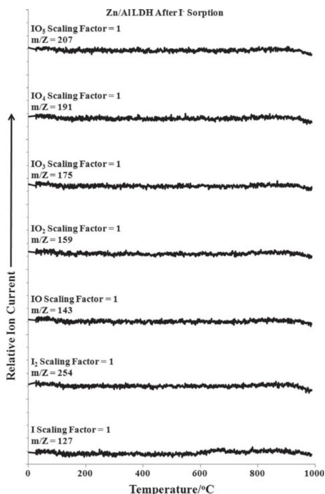
Fig. 7. Evolved gas mass spectrometry of Zn/Al LDH treated with I<sup>-</sup> solution gases absent.
