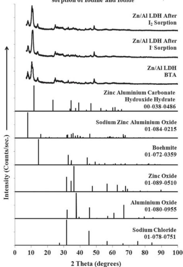
Fig. 2. Powder XRD pattern of Zn/Al LDH before thermal activation and after reformation in iodide or iodine solution with references.
