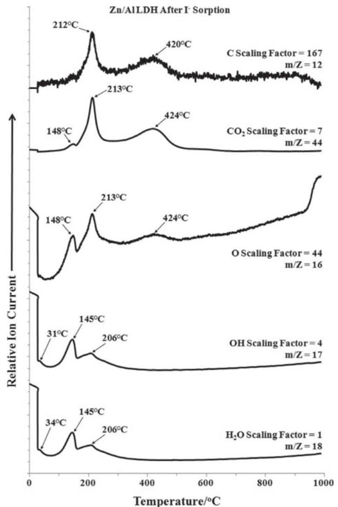
Fig. 6. Evolved gas mass spectrometry of Zn/Al LDH treated with I<sup>-</sup> solution gases detected.
