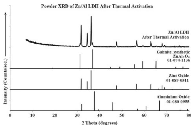
Fig. 3. Powder XRD pattern of Zn/Al LDH after thermal activation with references.
