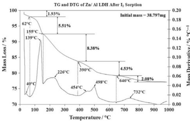
Fig. 5. TG and DTG curves of Zn/Al LDH after sorption of iodine.
