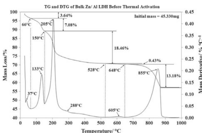
Fig. 1. TG and DTG curves of Zn/Al LDH before thermal activation or absorption experiments.
