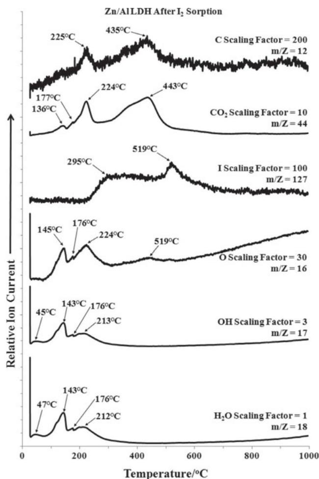
Fig. 8. Evolved gas mass spectrometry of Zn/Al LDH treated with I<sub>2</sub> solution.
