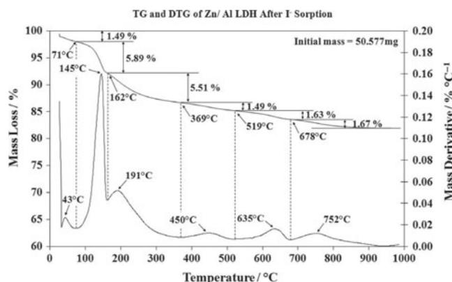
Fig. 4. TG and DTG curves of Zn/Al LDH after reformation in potassium iodide solution.
