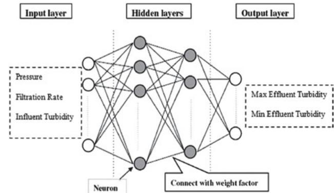
Fig. 2. Schematic architecture of artificial neural network in use.
