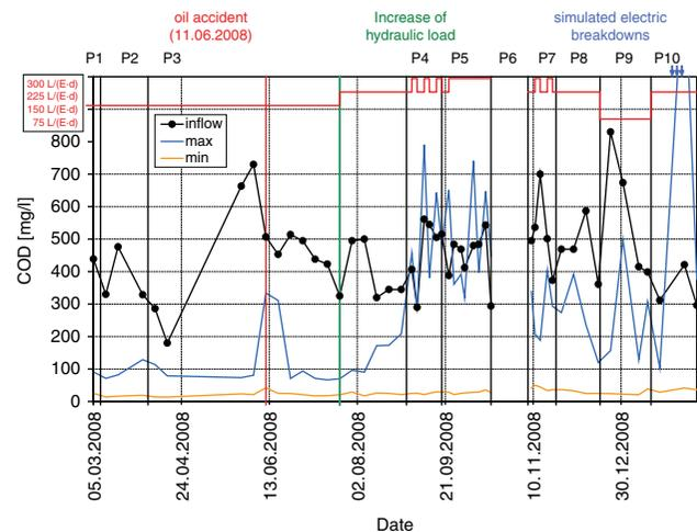
Fig. 2. COD curves for influent and the maximal and minimal effluent of all systems.
