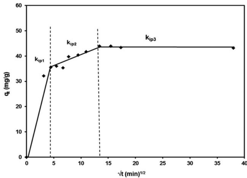
Fig. 5. Intra-particle diffusion kinetic model for  $\text{Co}^{2+}$  ion adsorption on the PSC obtained by the solid-combustion.
