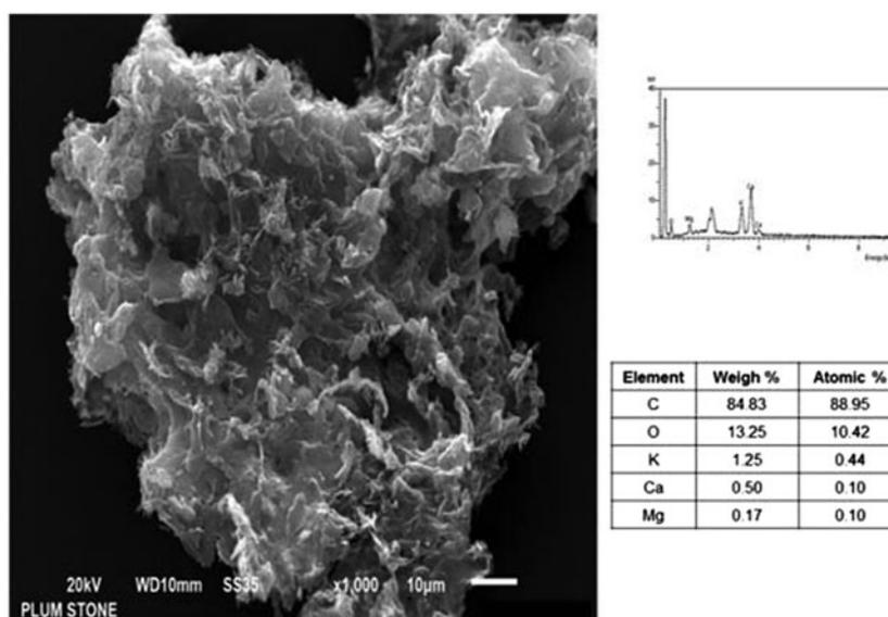
Fig. 2. SEM and EDS analysis of the PSC obtained by the solid-combustion process.
