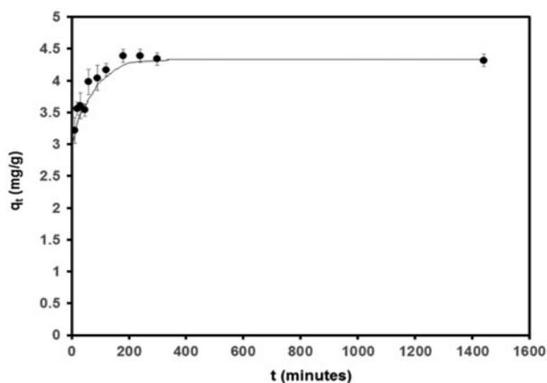
Fig. 4. Pseudo-second-order kinetic obtained by the non-linear method for the  $\text{Co}^{2+}$  ion adsorption on the as-prepared carbonaceous material.
