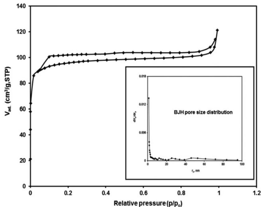
Fig. 3.  $N_2$  adsorption–desorption isotherm and inset BJH study of the PSC obtained by the solid-combustion process.
