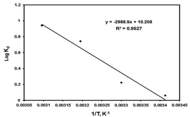
Fig. 9. Linear plot of  $\log K_d$  vs.  $1/T$  for the prepared carbonaceous adsorbent.
