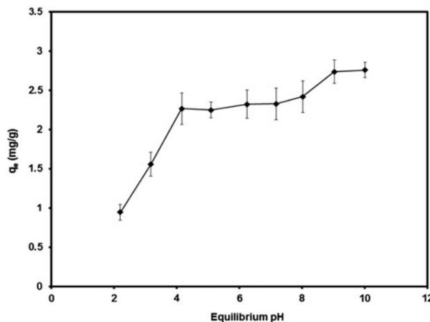
Fig. 7. pH effect of  $\text{Co}^{2+}$  ion adsorption on the carbonaceous adsorbent.
