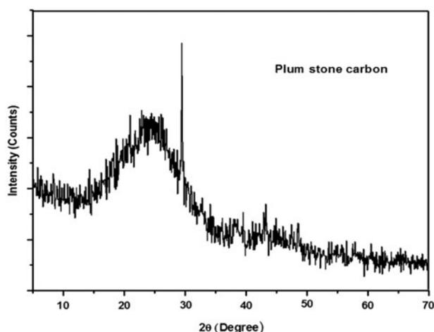
Fig. 1. XRD pattern of the PSC obtained by the solid-combustion process.
