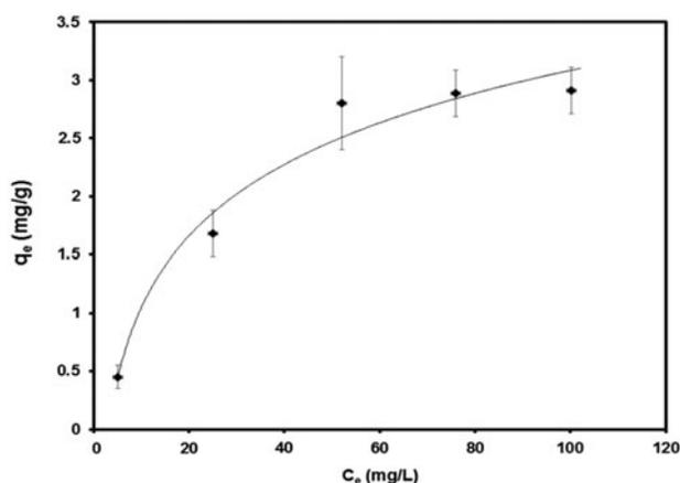
Fig. 6. Langmuir isotherm obtained by the non-linear method for  $\text{Co}^{2+}$  ion adsorption on the as-prepared carbonaceous material.
