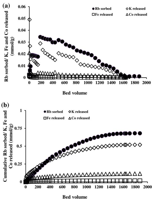
Fig. 6. (a) Individual and (b) cumulative Rb sorbed and K, Fe, Co released as a function of bed volumes in the column experiment (feed Rb concentration 5 mg/L, filtration velocity 2.5 m/h and bed height 12 cm).
