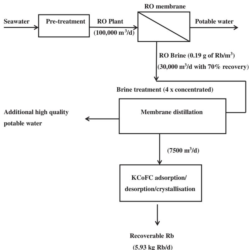
Fig. 8. Possible procedure for Rb recovery from SWROC.
