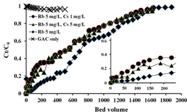
Fig. 5. Breakthrough curves for Rb sorption (filtration velocity  $2.5$  m/h, bed height  $12$  cm). The small graph within the large graph is an expanded version of the breakthrough curves up to  $250$  bed volumes.
