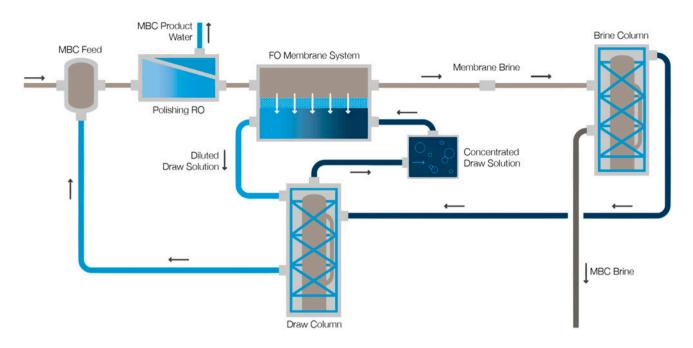
Fig. 6. Process flow schematic for the Changxing Power Plant MBC, including the preconcentration/polish RO membrane system, FO membrane system, and thermal draw recovery system. The primary difference between this process and the standard MBC is the preconcentration RO step used to treat the low TDS feedwater and improve overall process economics.
