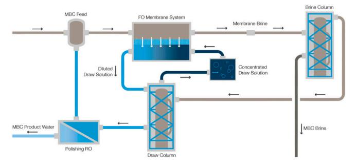
Fig. 2. Overall process flow schematic of the fully integrated MBC System.
