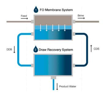
Fig. 1. High level view of a forward osmosis process, which relies on two primary systems: (1) the FO membrane system and (2) the draw recovery system.
