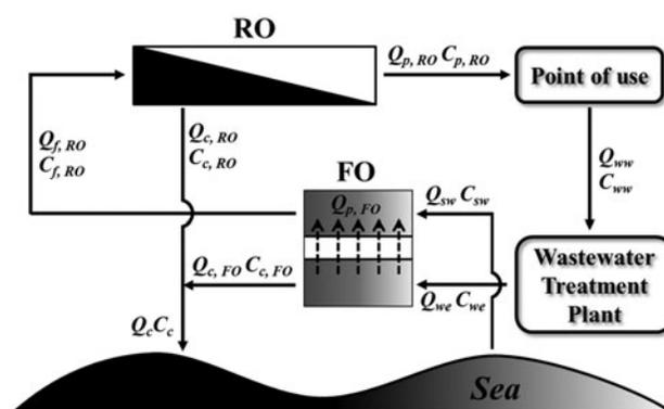
Fig. 1. The schematic of the FO-RO hybrid process. Notes:  $Q$ : flow rate,  $C$ : TDS concentration,  $f$ : feed,  $p$ : permeate,  $c$ : concentrate,  $sw$ : seawater,  $ww$ : wastewater,  $we$ : WWTP effluent.
