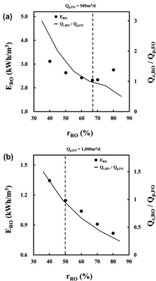
Fig. 3. The effect of the RO recovery on the RO energy consumption at 25°C for FO permeate flow rates: (a) 500 m<sup>3</sup>/d and (b) 1,000 m<sup>3</sup>/d.
