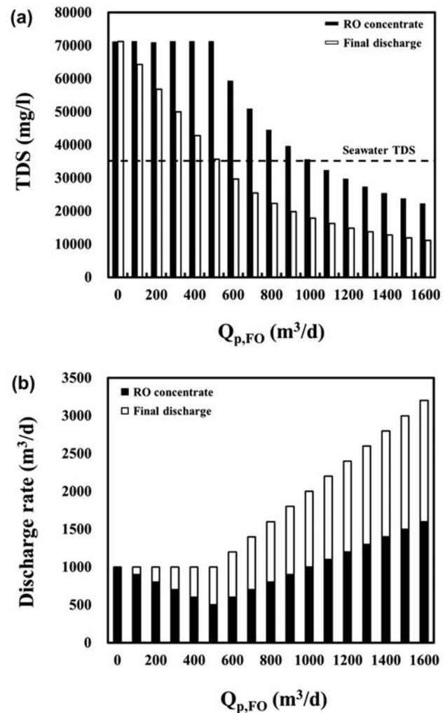
Fig. 5. The effect of the FO permeate flow rate on (a) the water quality and (b) flow rate of the final discharge of the FO-RO hybrid process.
