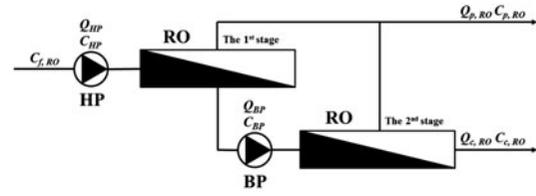
Fig. 2. The schematic of two-stage RO process to achieve high recovery (HP: high pressure pump, BP: booster pump).
