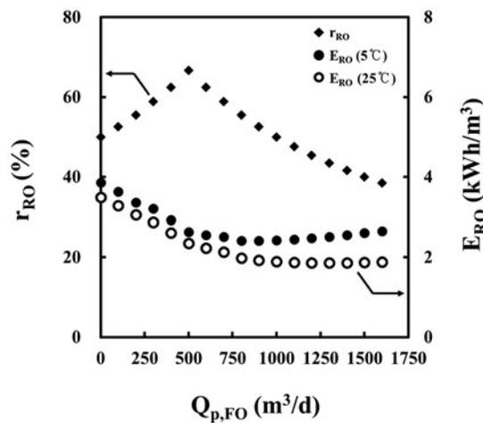
Fig. 4. The effect of the FO permeate flow rate on the optimal RO recovery and the RO energy consumption.
