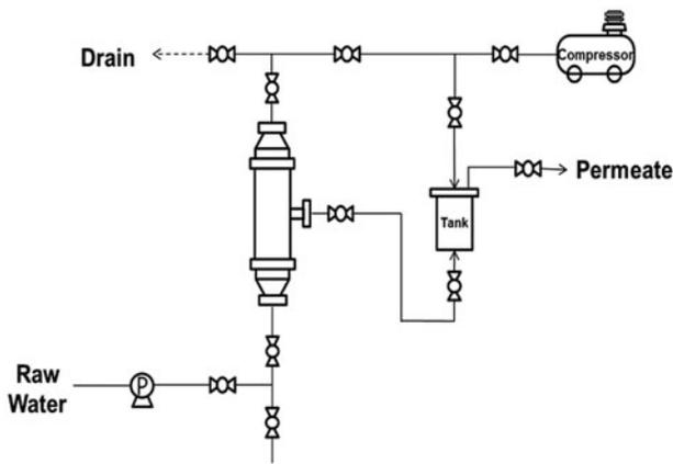
Fig. 1. Schematic diagram of the lab-scale ceramic MF system.
