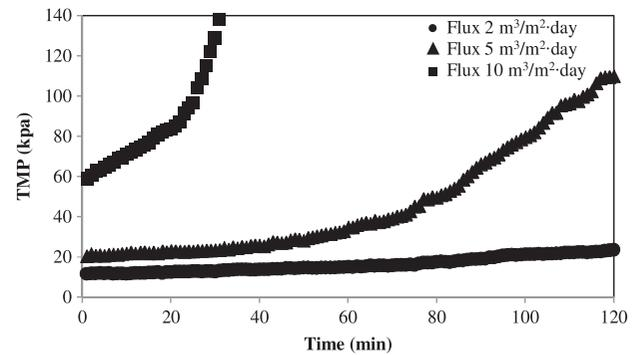
Fig. 5. TMP evolution at various membrane flux without coagulation.
