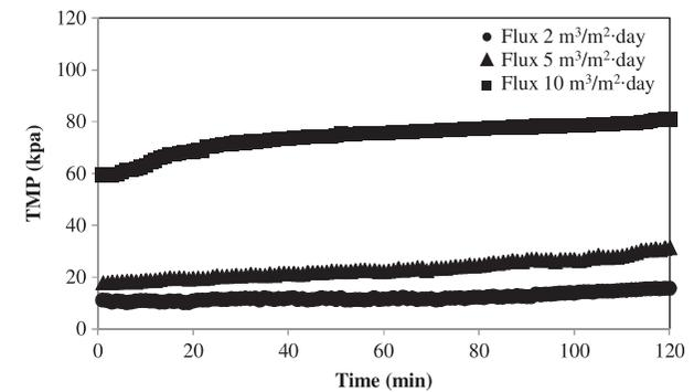
Fig. 6. TMP evolution at various membrane flux with coagulation (FeCl<sub>3</sub> 6 mg/L).
