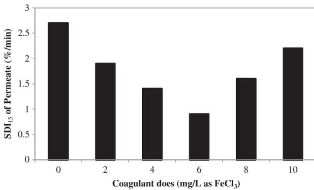
Fig. 2. Comparison of SDI<sub>15</sub> at different coagulation dose in ceramic MF system.
