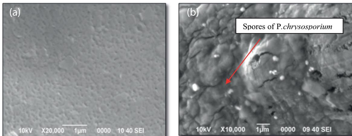
Fig. 1. SEM image: (a) plain beads and (b) beads with entrapped cells.
