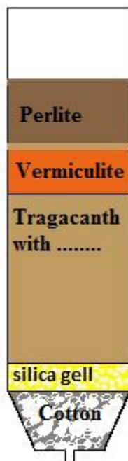
Fig. 1. Schematic view of biofilter construction.
