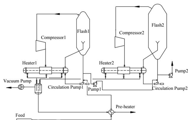
Fig. 1. Flow diagram of DEMVR system.
