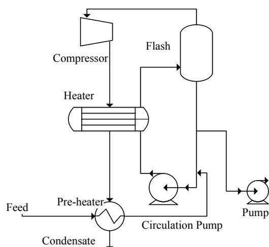
Fig. 2. Flow diagram of SEMVR system.
