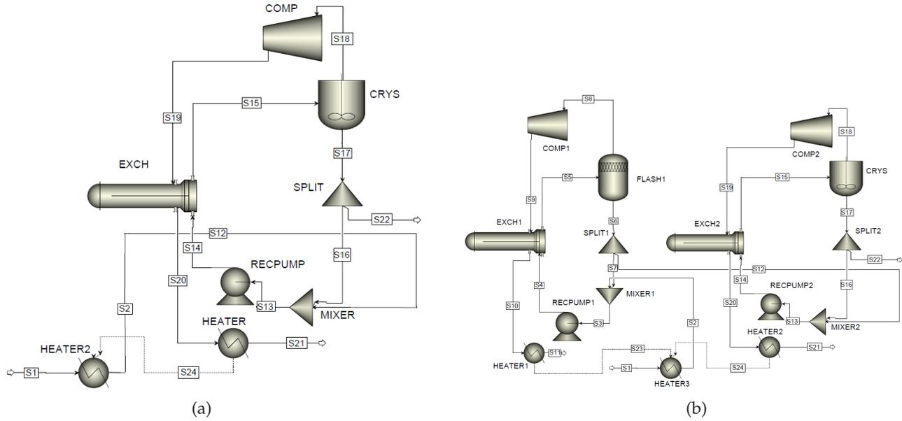
Fig. 3. Model of the system builds by Aspen Plus: (a) Model of SEMVR, and (b) Model of DEMVR.
