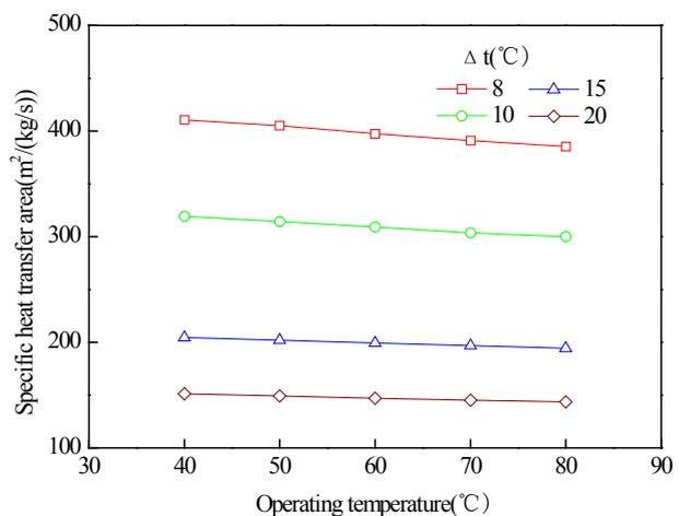
Fig. 8. Variation in specific heat transfer area of the system as a function of operating temperature and the temperature difference.
