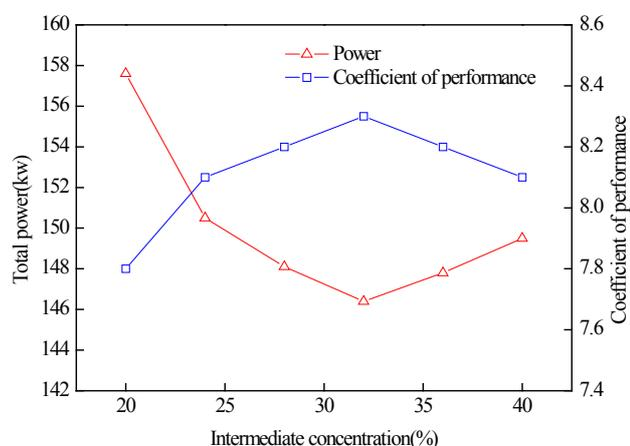
Fig. 4. Effect of the intermediate concentration on the total power and performance coefficient of system.
