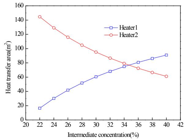
Fig. 6. Variation of the heat-transfer area as a function of the intermediate concentration.
