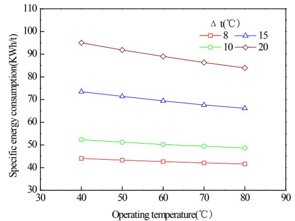
Fig. 7. Variation in specific energy consumption of the system as a function of the temperature difference and operating temperature.
