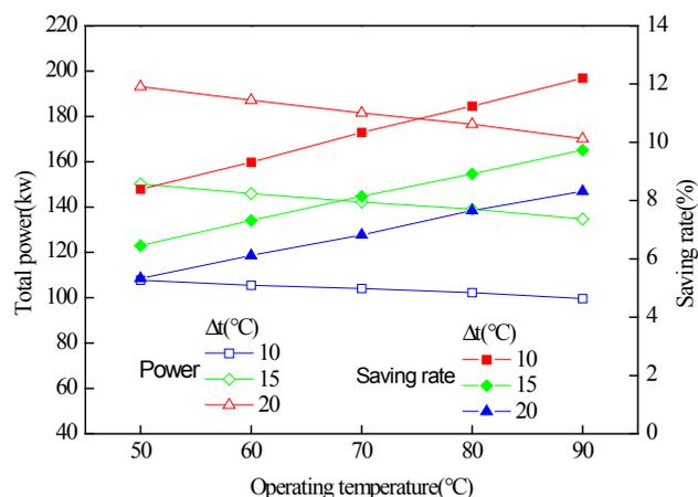
Fig. 5. Effect of operating temperature and temperature difference on the total power and saving rate.
