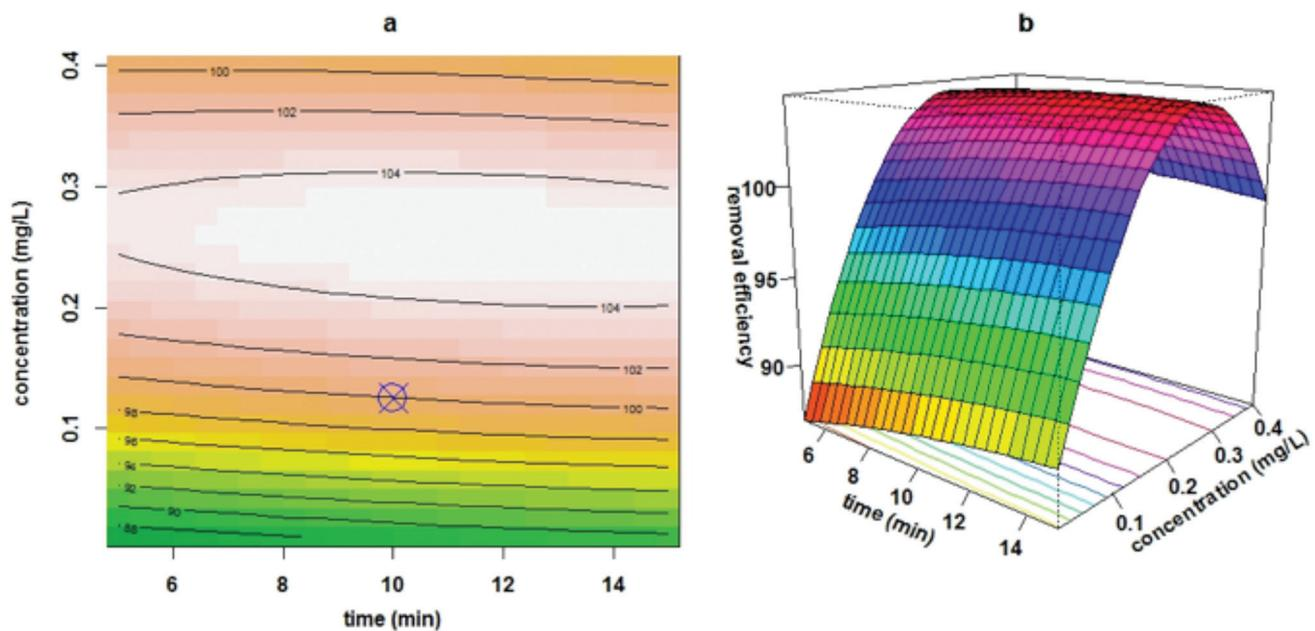
Fig. 5. Contour (a) for respective three dimensional curve, and (b) for interactive effect of time and concentration on disinfection efficiency of NaOCl.
