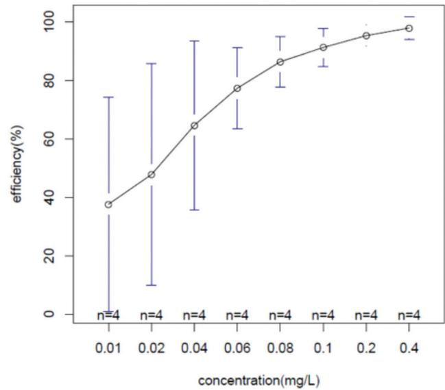
Fig. 1. Mean plot of disinfection efficiency at different concentrations of NaOCl.
