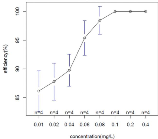
Fig. 2. Mean plot of disinfection efficiency at different concentrations of NaDCC.
