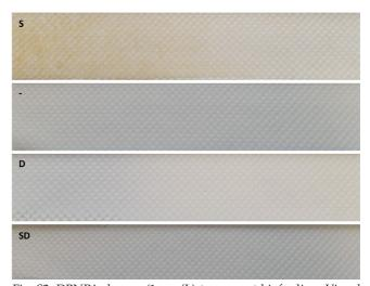
Fig. S2. DBNPA dosage (1 mg/L) to prevent biofouling. Visual observation of the accumulated material on the membrane and feed spacer in the MFS-units, directly prior sampling for ATP and TOC analysis. S substrate only, – negative control, D DBN-PA only and SD.
