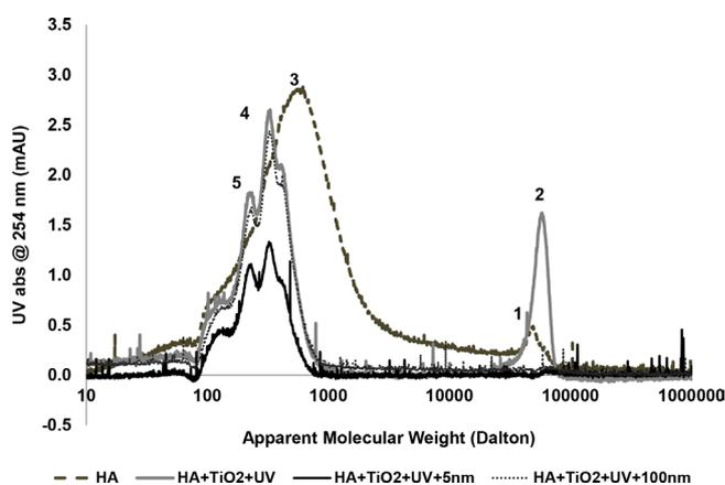
Fig. 7. LC analysis of HA at different stages of treatment (HA concentration: 20 mg/L,  $\text{TiO}_2$  = 0.5 g/l, pH: 7.5; UV intensity: 3.4 mW/cm<sup>2</sup>).
