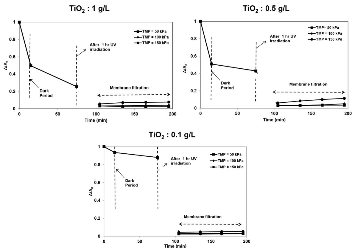
Fig. 6. Reduction in UV absorbance of the photocatalytic-UF ceramic membrane integrated system under different TMP and various  $\text{TiO}_2$  concentrations (HA concentration: 20 mg/L, pH: 7.5; UV intensity: 3.4 mW/cm<sup>2</sup>).
