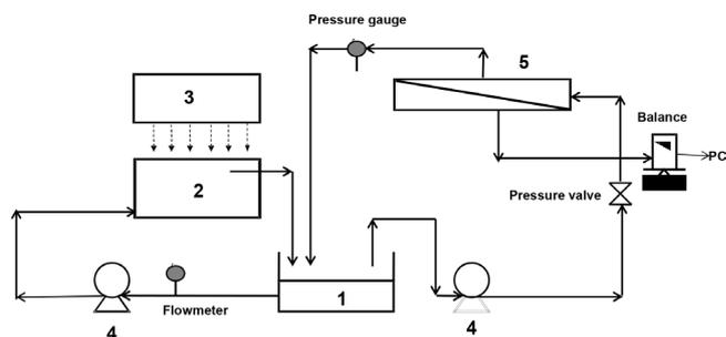
Fig. 1. Schematic diagram of the photocatalysis/ ceramic membrane system. (1) Feed tank (2) Photoreactor (3) UV lamp (4) Peristaltic pump (5) Ceramic membrane.
