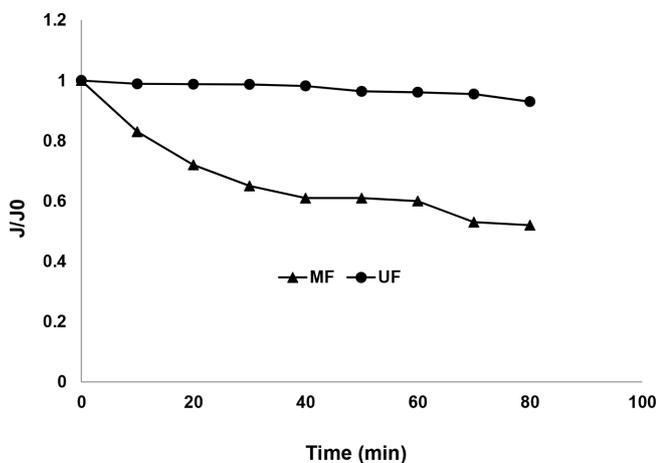
Fig. 2. Normalised flux vs time for different pore sizes of ceramic membranes ( $\text{TiO}_2$  concentration:  $0.5 \text{ g}/\text{L}$ , HA concentration:  $20 \text{ mg}/\text{L}$ , TMP:  $100 \text{ kPa}$  (UF) &  $20 \text{ kPa}$  (MF),  $\text{pH}$ :  $7.5$ ; UV intensity:  $3.4 \text{ mW}/\text{cm}^2$ ).
