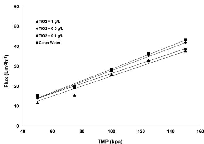
Fig. 4. Effect of TMP on the UF permeate flux under different TiO<sub>2</sub> concentrations (HA concentration: 20 mg/L, pH: 7.5; UV intensity: 3.4 mW/cm<sup>2</sup>).
