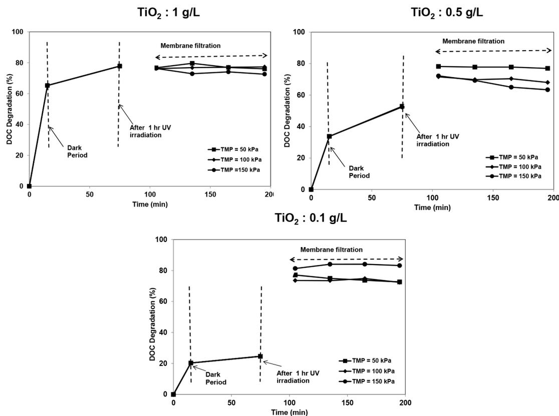
Fig. 5. DOC removal efficiency of the photocatalytic–ceramic ultrafiltration membrane integrated system under different TMP and various TiO<sub>2</sub> concentrations (HA concentration: 20 mg/L, pH: 7.5; UV intensity: 3.4 mW/cm<sup>2</sup>).
