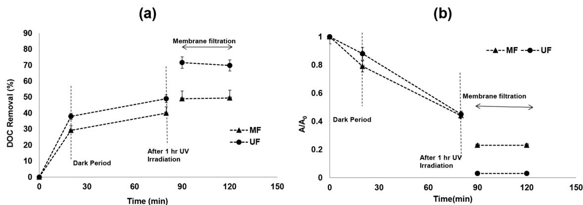
Fig. 3. (a) Dissolved organic carbon (DOC) removal efficiency; (b) reduction in UV absorbance of the photocatalytic–ceramic membrane integrated system for different pore sizes (HA concentration: 20 mg/L, TiO<sub>2</sub> concentration: 0.5 g/L, TMP: 100 kPa (UF) & 20 kPa (MF), pH: 7.5; UV intensity: 3.4 mW/cm<sup>2</sup>).
