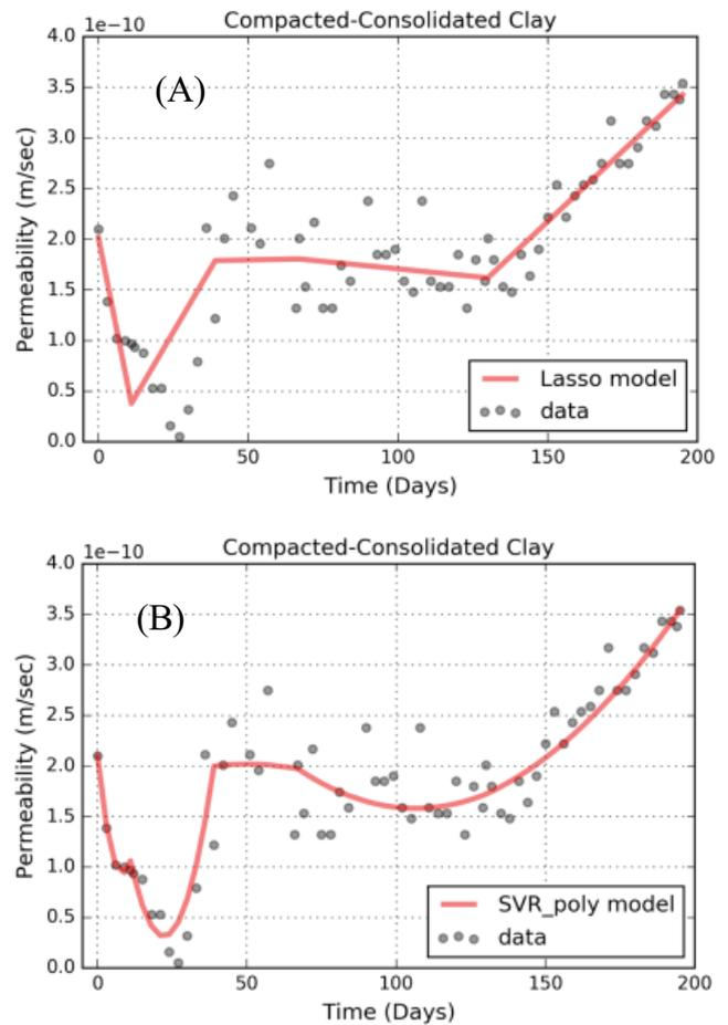
Fig. 3. Lasso regression model (A) and SVR model (B) for compacted-consolidated clay sample.
