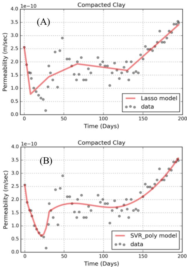
Fig. 2. Lasso regression model (A) and SVR model (B) for compacted contaminated clay sample.
