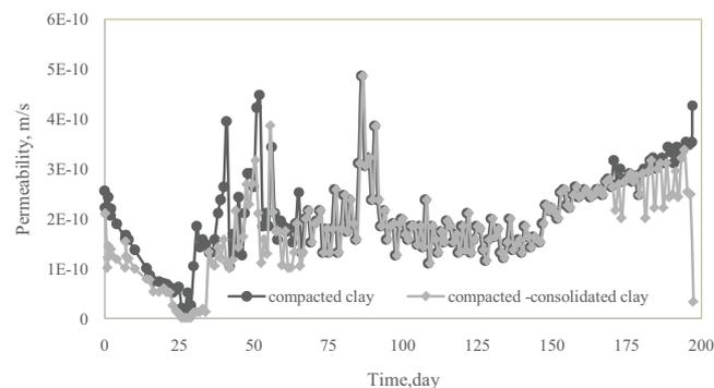
Fig. 4. Permeability changes in compacted clay and compacted–consolidated clay.
