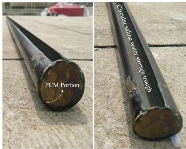
Fig. 10. Circular water storage trough with PCM.
