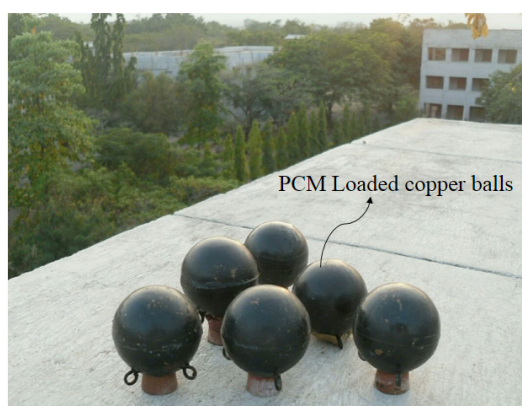
Fig. 5. The PCM loaded copper balls with rubber cork.
