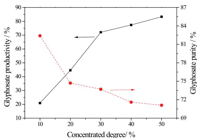
Fig. 12. Gly productivity and purity with respect to the concentrated degree of the residual solution.
