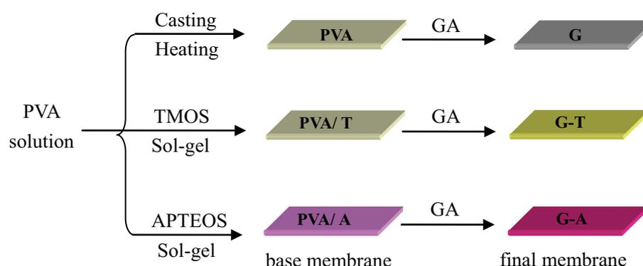
Fig. 1. Preparation procedures for membranes G, G-T and G-A.
