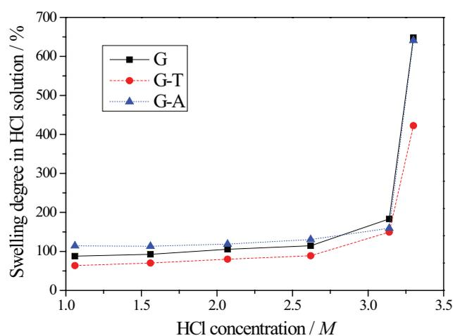
Fig. 6. Swelling degrees in HCl solutions (1.1–3.3 M) for 48 h.
