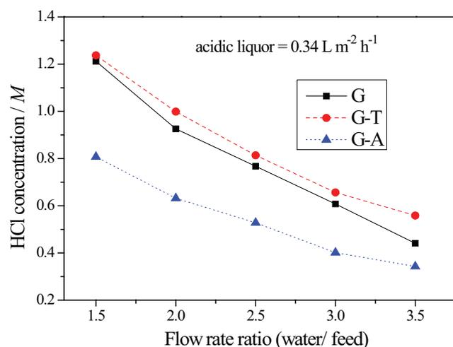
Fig. 10. (a) Recovered HCl concentrations ( $C_{d-H}$ ) with respect to the flow rate ratio.
