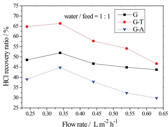
Fig. 9. (a) HCl recovery ratio ( $R_H$ ) with respect to the flow rate of water or acidic liquor.
