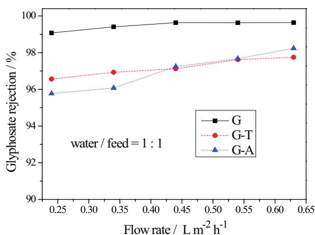
Fig. 9. (b) Gly rejection ( $\eta_{Gly}$ ) with respect to the flow rate of water or acidic liquor.
