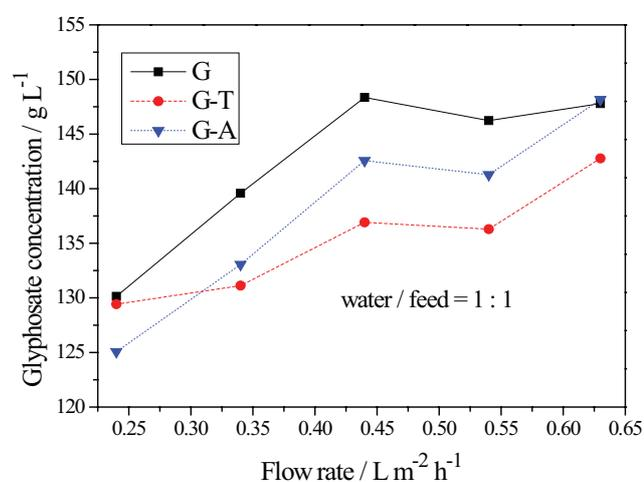
Fig. 8. (b) Residual Gly concentrations with respect to the flow rate of water or acidic liquor.
