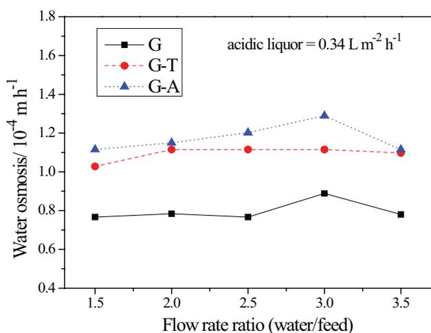
Fig. 7. (b)  $U_{H_2O}$  with respect to the flow rate ratio of water/feed.
