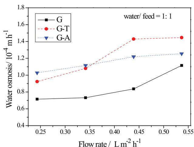
Fig. 7. (a) Water osmosis coefficients ( $U_{H_2O}$ ) with respect to the flow rate of water or acidic liquor.
