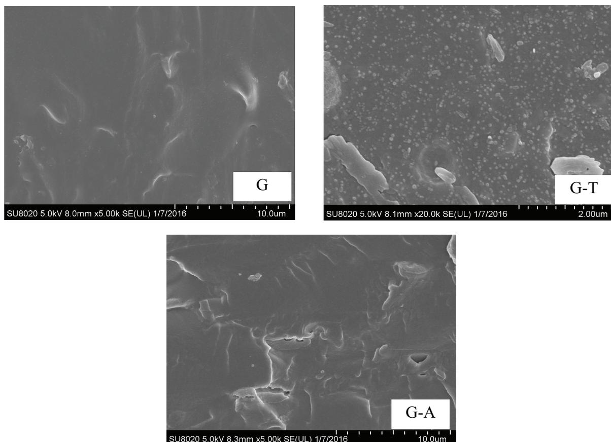
Fig. 4. The SEM images of membrane cross-sections.
