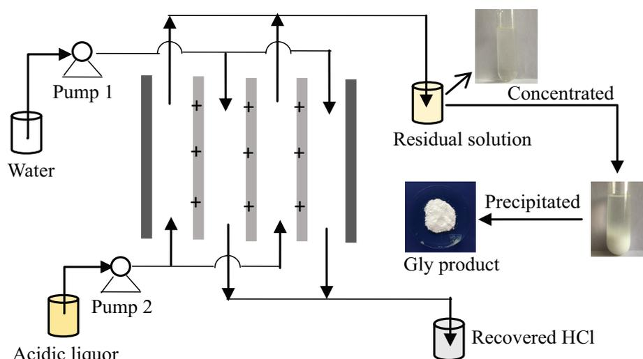
Fig. 2. Continuous diffusion dialysis (DD) for separating the acidic liquor to obtain recovery HCl and Gly product.
