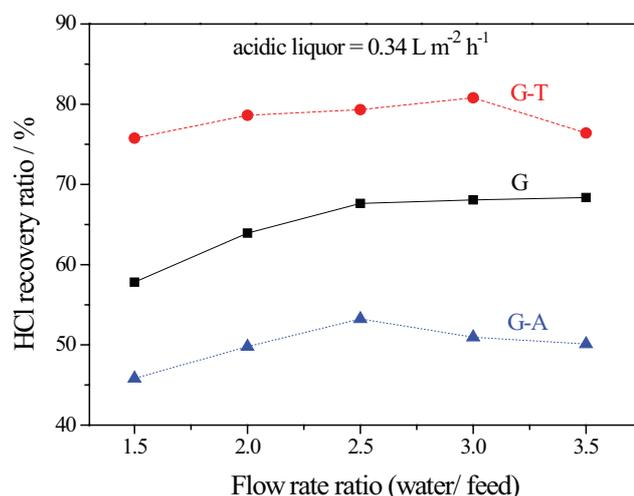
Fig. 11. (a) HCl recovery ratio ( $\eta_H$ ) with respect to the flow rate ratio.
