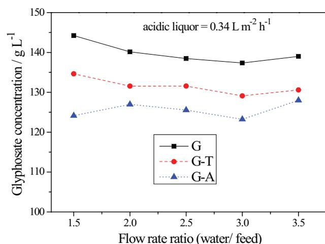
Fig. 10. (b) Residual Gly concentrations ( $C_{\text{res-Gly}}$ ) with respect to the flow rate ratio.
