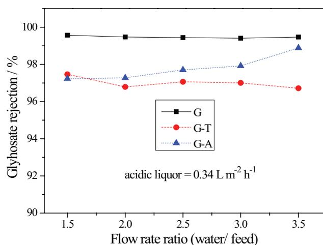
Fig. 11. (b) Gly rejection ( $\eta_{\text{Gly}}$ ) with respect to the flow rate ratio.
