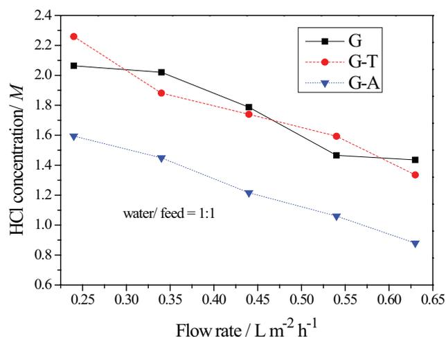
Fig. 8. (a) Recovered HCl concentrations with respect to the flow rate of water or acidic liquor.
