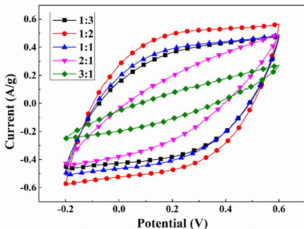
Fig. 5. CV curves of the PPy/CNT electrodes fabricated with different mass ratio of PVDF and graphite powder at the scanning rate of 5 mV/s in 1 M NaCl solution.
