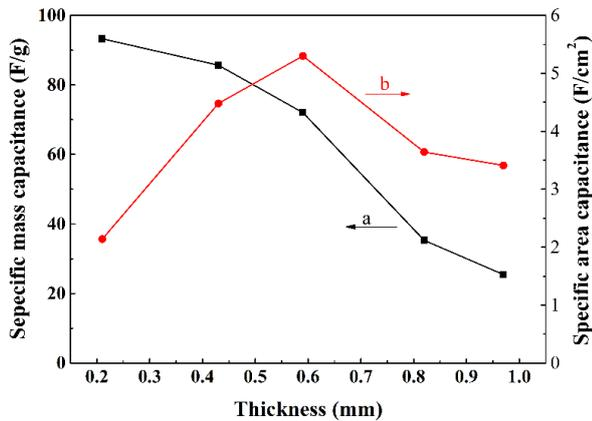
Fig. 8. The specific mass capacitance and the specific area capacitance of the electrodes with different thickness.
