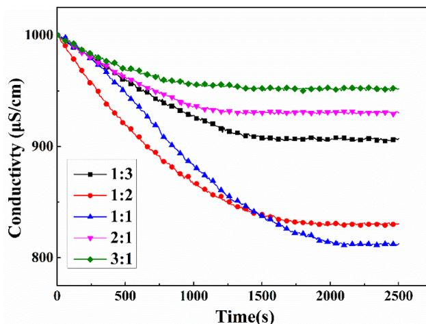
Fig. 6. Saturated adsorption curves of the PPy/CNT electrodes fabricated with different mass ratio of PVDF and conductive graphite powder at a working voltage of 1.4 V in NaCl solution.
