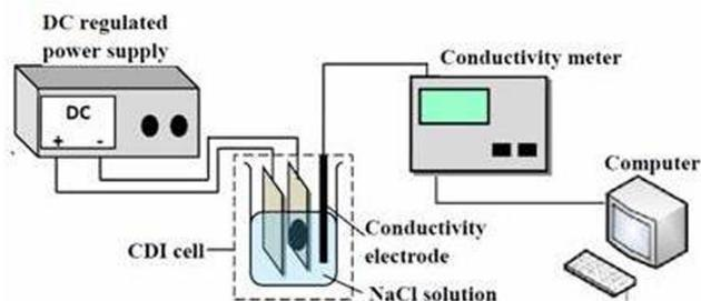
Fig. 2. Schematic diagram of the CDI desalinating system.
