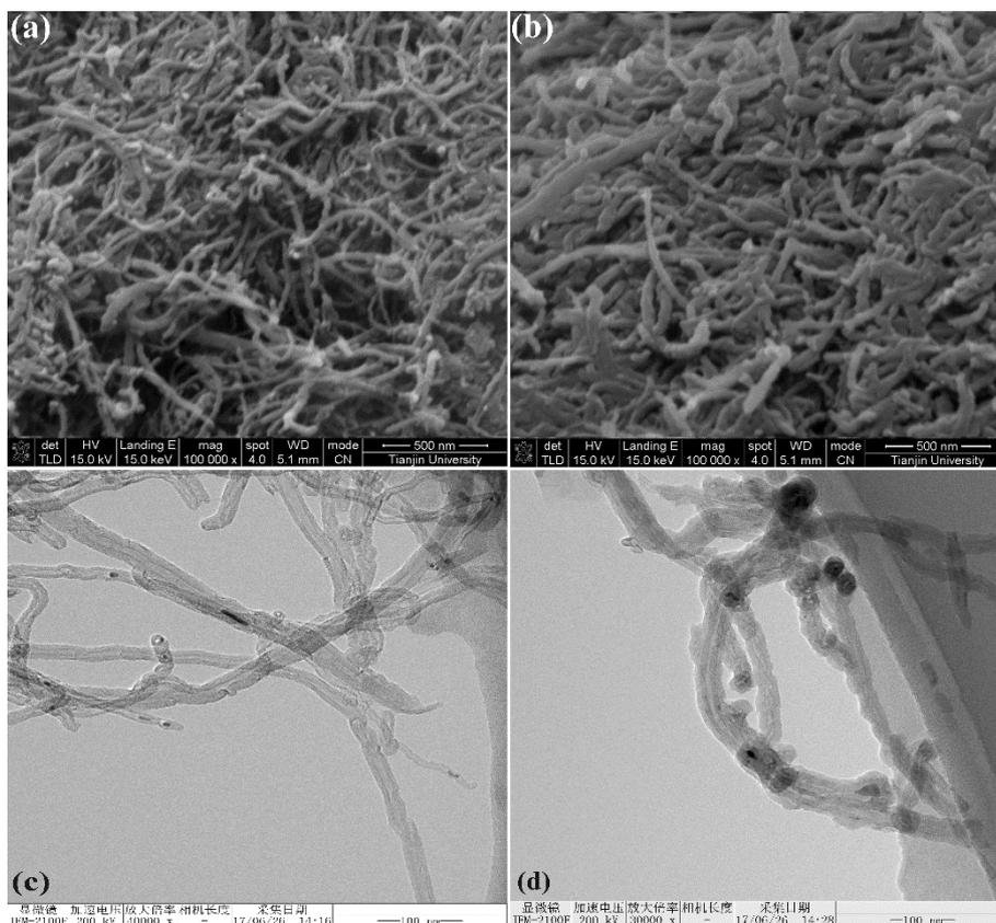
Fig. 10. FE-SEM and TEM images of CNT (a, c) and PPy/CNT (b, d) after applying the moulding pressure of 25 MPa.
