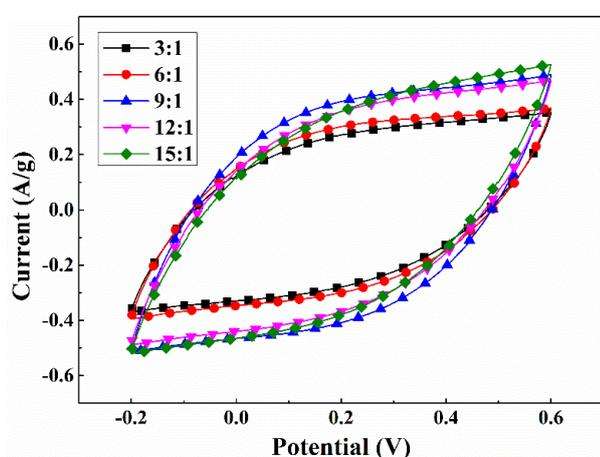
Fig. 3. CV curves of the PPy/CNT electrodes fabricated with different mass ratio of PPy/CNT and PVDF at the scanning rate of 5 mV/s in 1 M NaCl solution.
