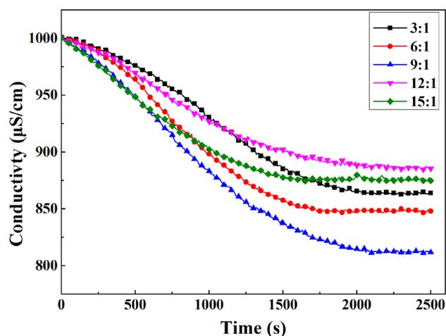
Fig. 4. Saturated adsorption curves of the PPy/CNT electrodes fabricated with different mass ratio of PPy/CNT and PVDF at a working voltage of 1.4 V.
