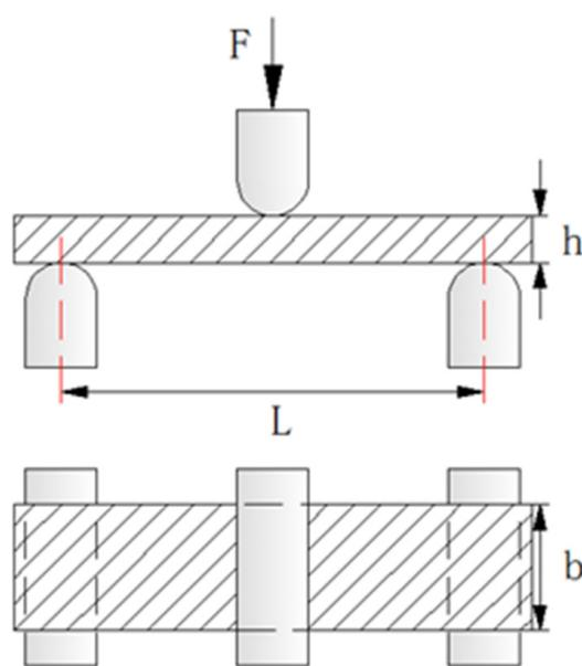
Fig. 1. Schematic diagram of three-point bending test.
