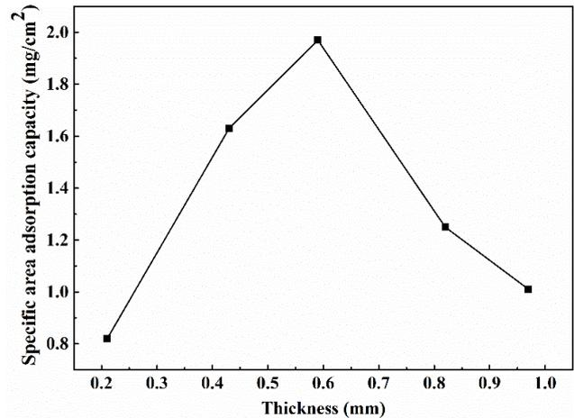
Fig. 9. The change of specific area adsorption capacity of electrodes with different thickness.
