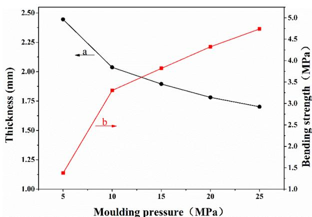
Fig. 11. The change of thickness (a) and bending strength (b) of electrodes fabricated by different moulding pressure.
