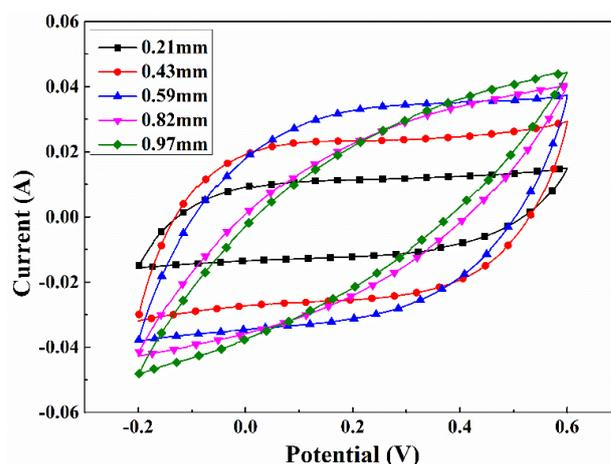
Fig. 7. CV curves of the electrodes with different thickness at the scanning rate of 5 mV/s in 1 M NaCl solution.
