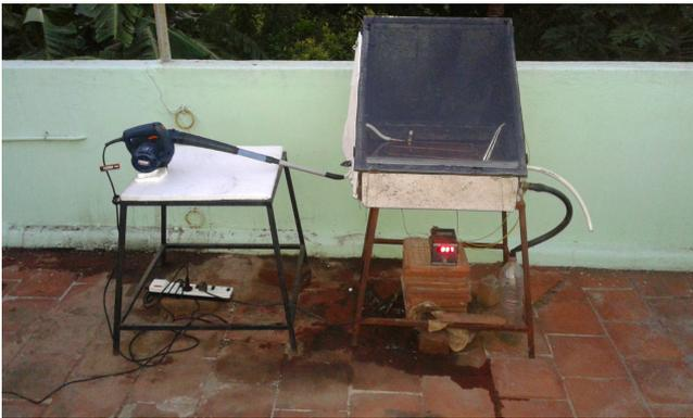
Fig. 3. Photographic view of the still with air blower.
