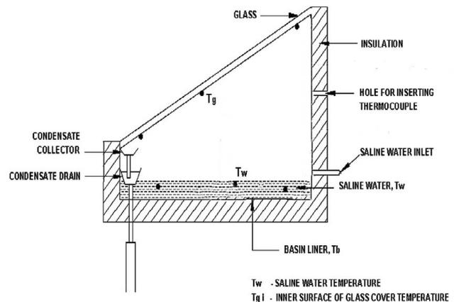
Fig. 1. Schematic diagram of the single-slope single-basin solar still.
