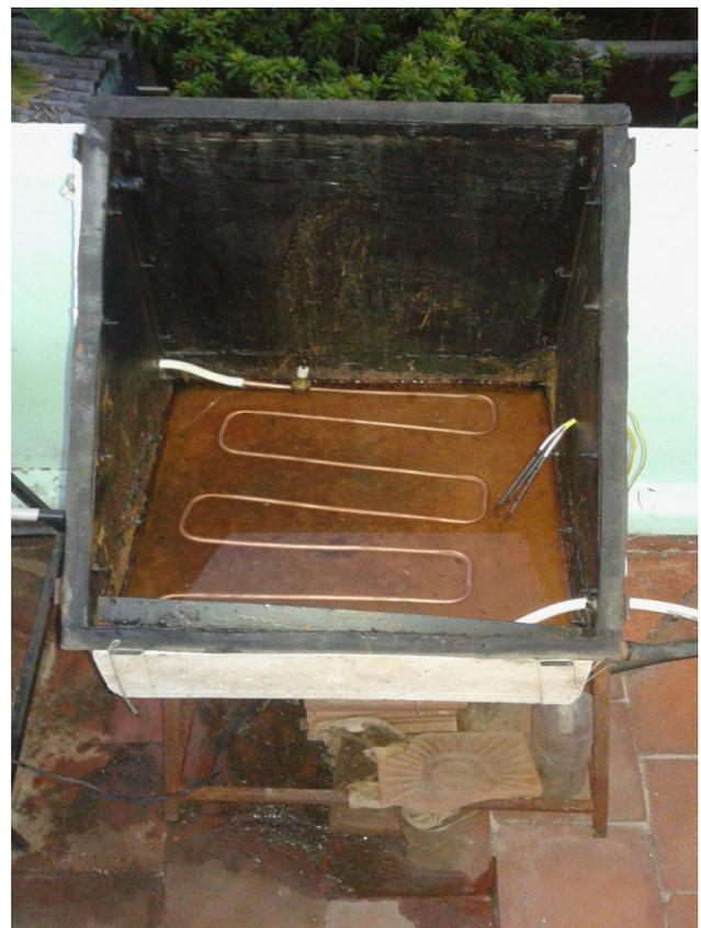
Fig. 2. Photographic view of the copper pipe placed in the still.
