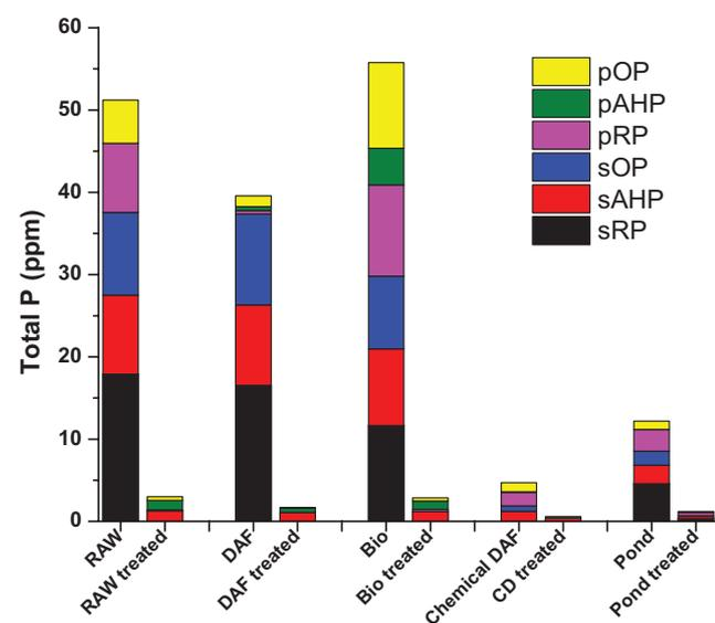
Fig. 5. Distribution and comparison of P species in wastewaters before and after Al-MNP treatment for the samples collected at the different stages of wastewater treatment.
