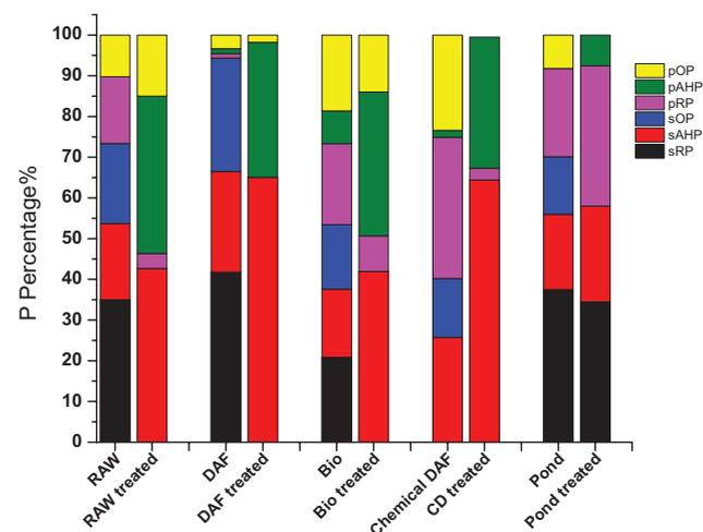
Fig. 6. Percentage distribution of each P species in wastewaters before and after Al-MNP treatment for the samples collected at the different stages of wastewater treatment.
