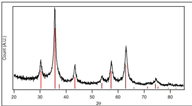
Fig. 3. X-ray diffraction patterns of pure and Al-doped magnetite. The locations and intensities of peaks are in agreement with the standard magnetite (red lines) JCPDS card (card no. 19-0629).
