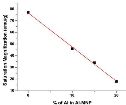
Fig. 4. Magnetic moment measurements for pure and Al-doped MNP.
