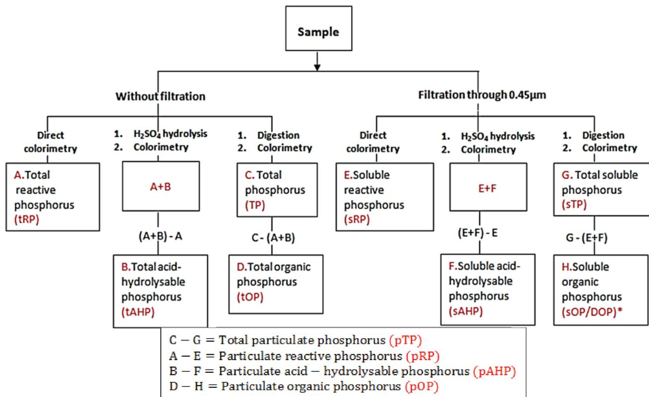
Fig. 2. Analytical methods for the determination of various P fractions.
