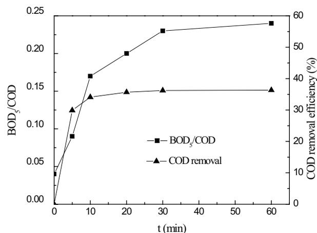
Fig. 4. Effect of  $ClO_2$  oxidation time on the biodegradability and  $COD$  removal of OTC wastewater ( $ClO_2$  0.2  $mM$ ,  $pH 7.0$ ,  $BOD_5$  test at  $pH 7$ ).
