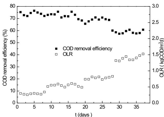
Fig. 7. Effects of OLR on BAC performance under HRT of 8 h and ClO<sub>2</sub> dosage of 78.9 mg/L.
