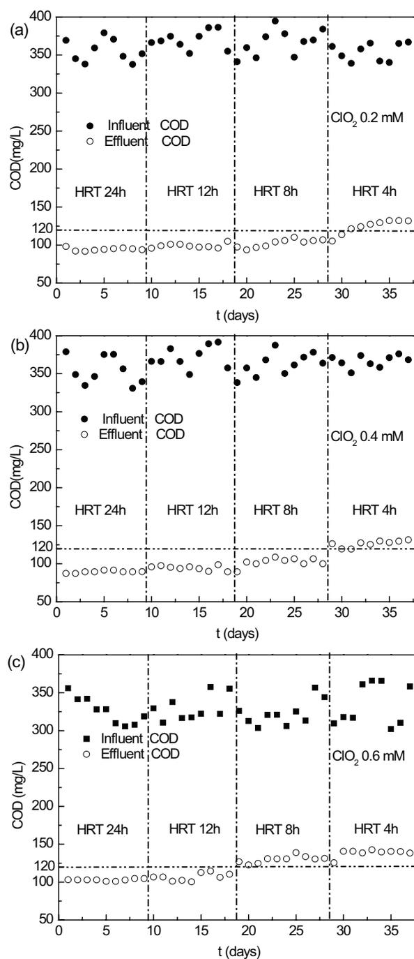
Fig. 6. COD removal by BAC reactor combined with (a) 0.2 mM  $\text{ClO}_2$  pre-oxidation, (b) 0.4 mM  $\text{ClO}_2$  pre-oxidation and (c) 0.6 mM  $\text{ClO}_2$  pre-oxidation as a function of HRT under DO 3 mg/L and OLR 0.25 kg COD/m<sup>3</sup>·d.
