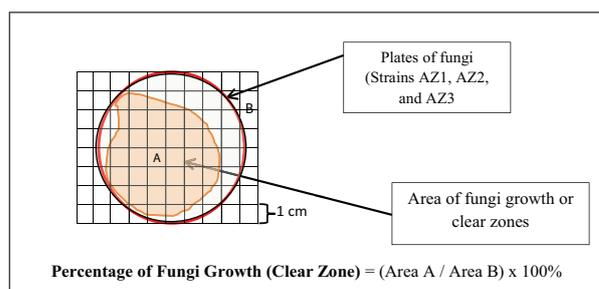
Fig. 1. Grid method for determining the percentage of clear zones appeared.
