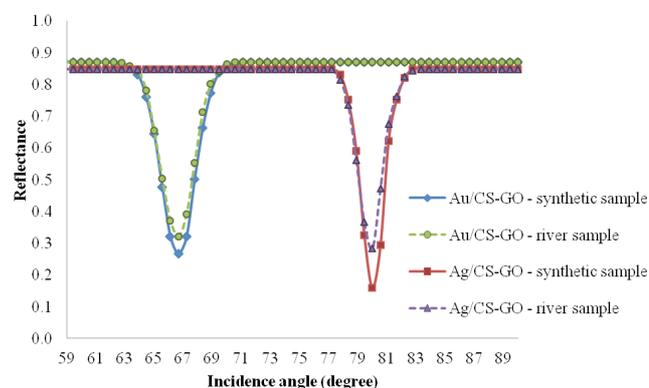
Fig. 6. The SPR curves of the (a) Au/CS-GO and (b) Ag/CS-GO thin films for water samples from the Saigon River.
