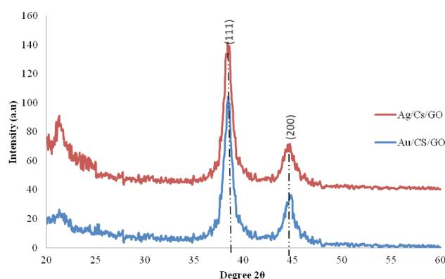
Fig. 3. The X-ray diffraction (XRD) patterns of the Au/CS-GO and Ag/CS-GO thin films.
