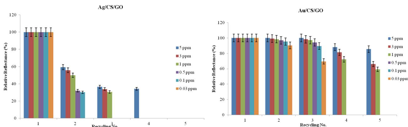
Fig. 5. The reusability of the (a) Au/CS-GO and (b) Ag/CS-GO thin films.
