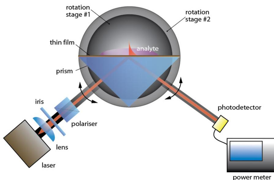
Fig. 2. SPR experimental setup (Adapted from [27]).
