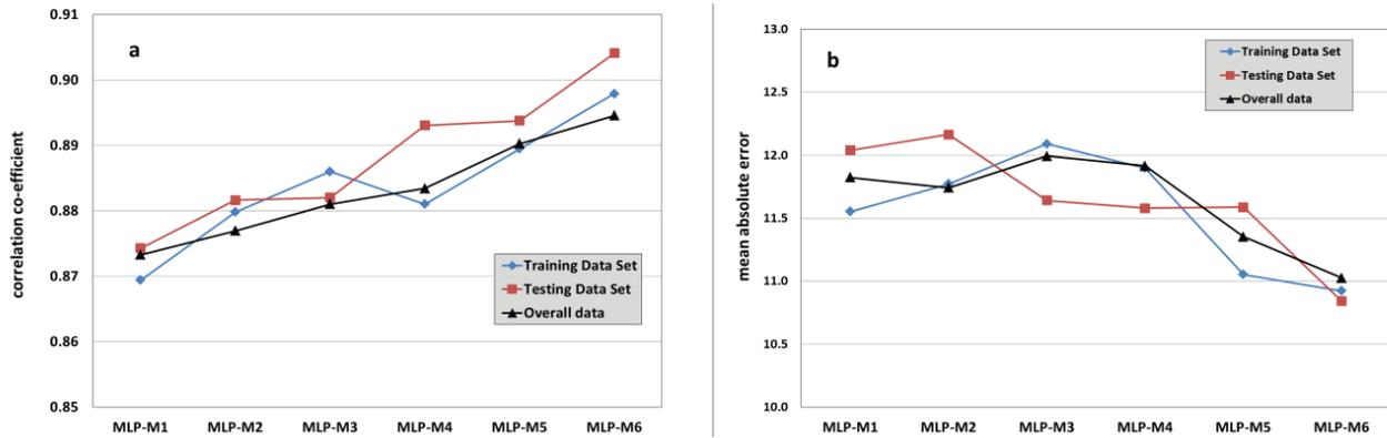
Fig. 5. Performance values of MLP models: (a) correlation co-efficient and (b) mean absolute error.
