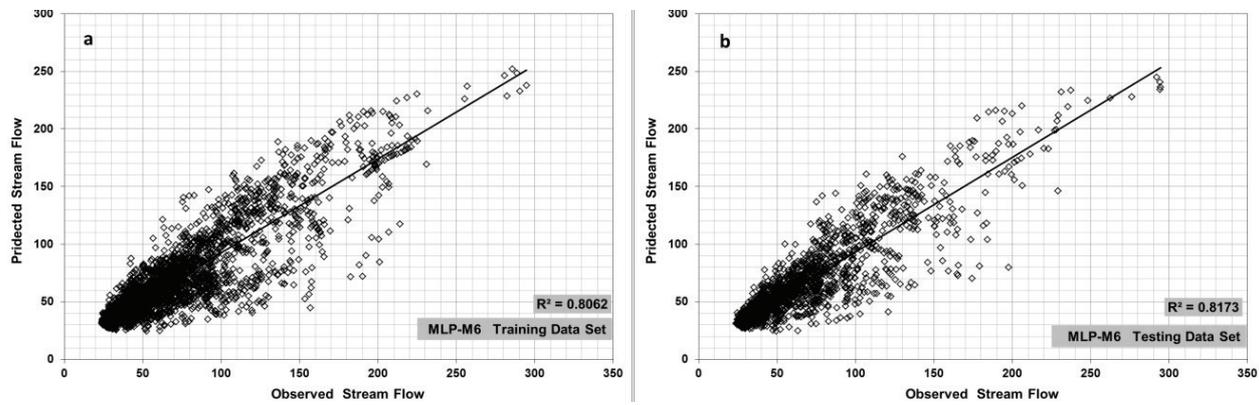
Fig. 6. Correlation between the observed and predicted hourly stream flow by M6-MLP model: (a) training data set, and (b) Testing data set.
