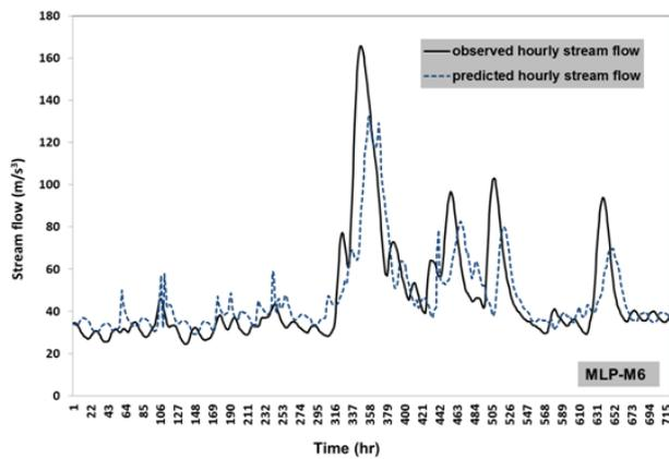
Fig. 7. Comparison between the observed and predicted hourly stream flow using the M6-MLP model.
