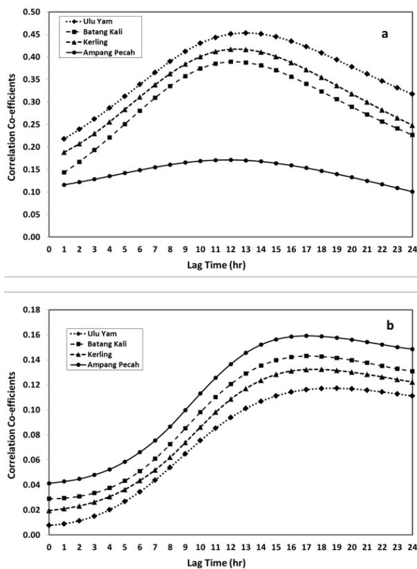
Fig. 4. Correlation co-efficient between hourly stream flow records of downstream station and hourly records of upstream station: (a) Water level station, and (b) Rainfall station.
