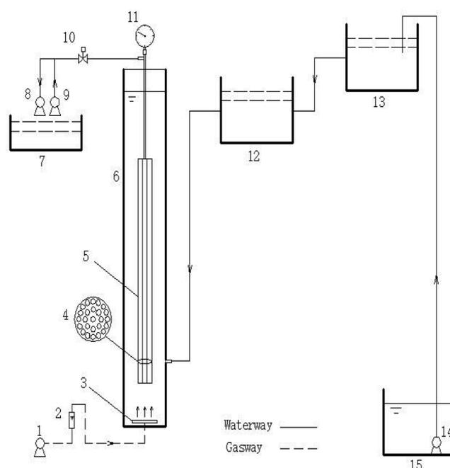
Fig. 1. The experimental facility (1 – Air pump; 2 – Gas flow meter; 3 – Air diffuser; 4 – Cross section; 5 – Membrane; 6 – Bio-reactor; 7 – Sink tank; 8 – Suction pump; 9 – Backwash pump; 10 – Relays; 11 – Vacuum gauge; 12 – Constant level tank; 13 – High water tank; 14 – Submersible pump; 15 – Water distribution tank).
