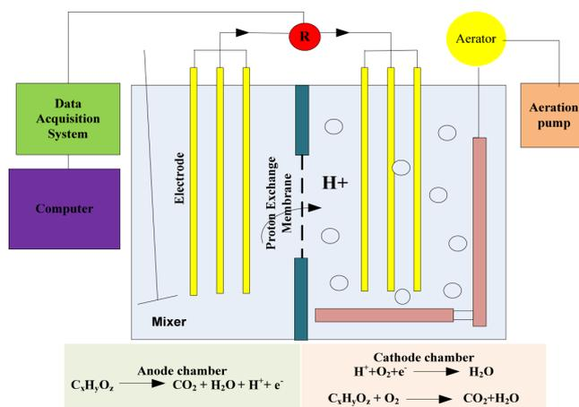
Fig. 1. A schematic view of the utilized laboratory set-up and its related reactions.
