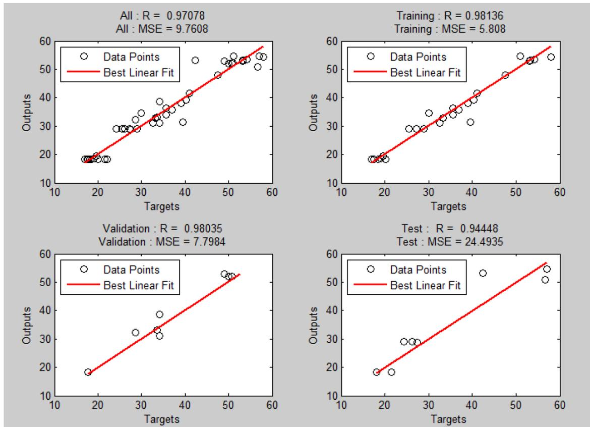
Fig. 8. The correlation coefficients (R) for training, validating, and testing subset data considering the VSS removal efficiency.
