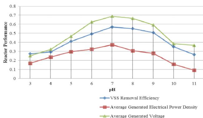
Fig. 3. the effect of the pH value on the reactor performance (T = 35°C; the initial VSS of the waste activated sludge = 4400 ± 100 mg/L).
