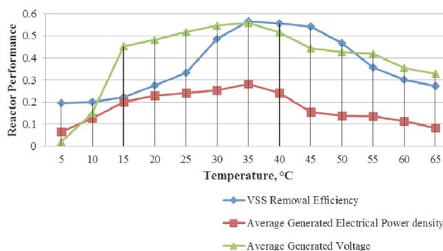
Fig. 2. the effect of the temperature on the reactor performance (pH = 7; the initial VSS of the waste activated sludge =  $4400 \pm 100$  mg/L)
