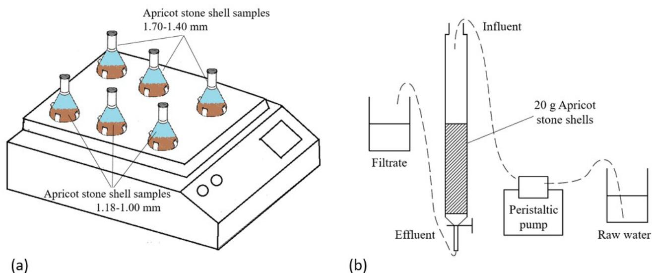
Fig. 2. The experimental setups for organic matter release tests (a) constant volume container experiments and (b) fixed bed filtration experiments.
