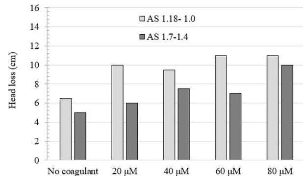
Fig. 9. Total head loss across the bed.
