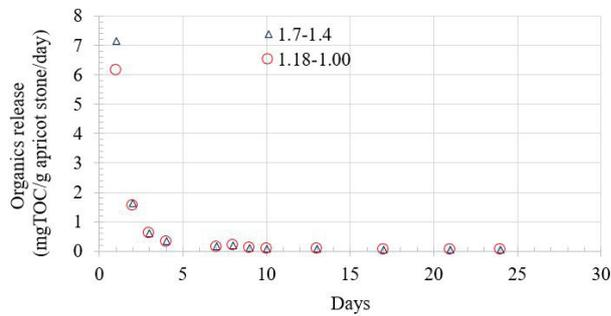
Fig. 6. Total organic carbon content in samples contacting with apricot stone particles at constant temperature and constant volume.
