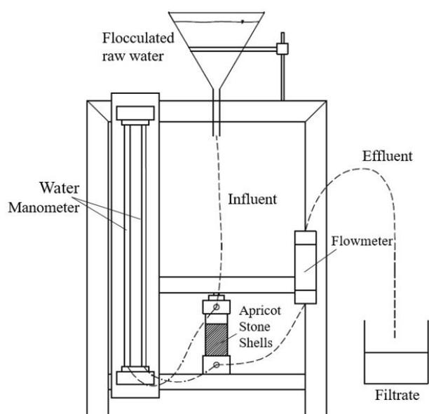
Fig. 3. The experimental setup used for filterability tests.
