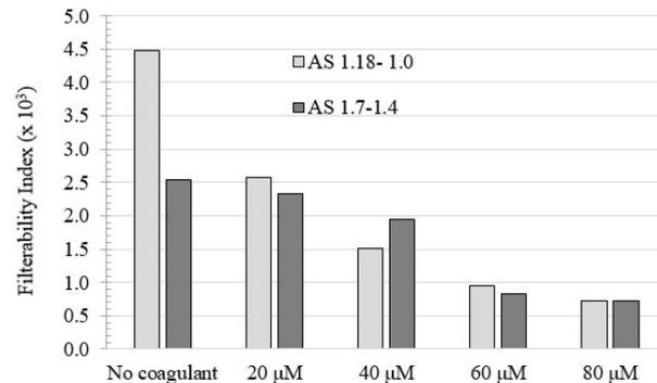
Fig. 10. Filterability Index (FI).
