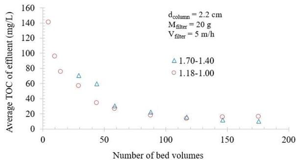
Fig. 7. Total organic carbon content in samples taken from the effluent of filter bed containing apricot stone shells.
