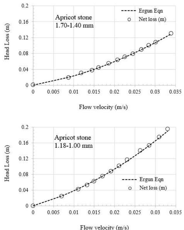
Fig. 5. Fixed-bed head loss data for apricot stone fractions.
