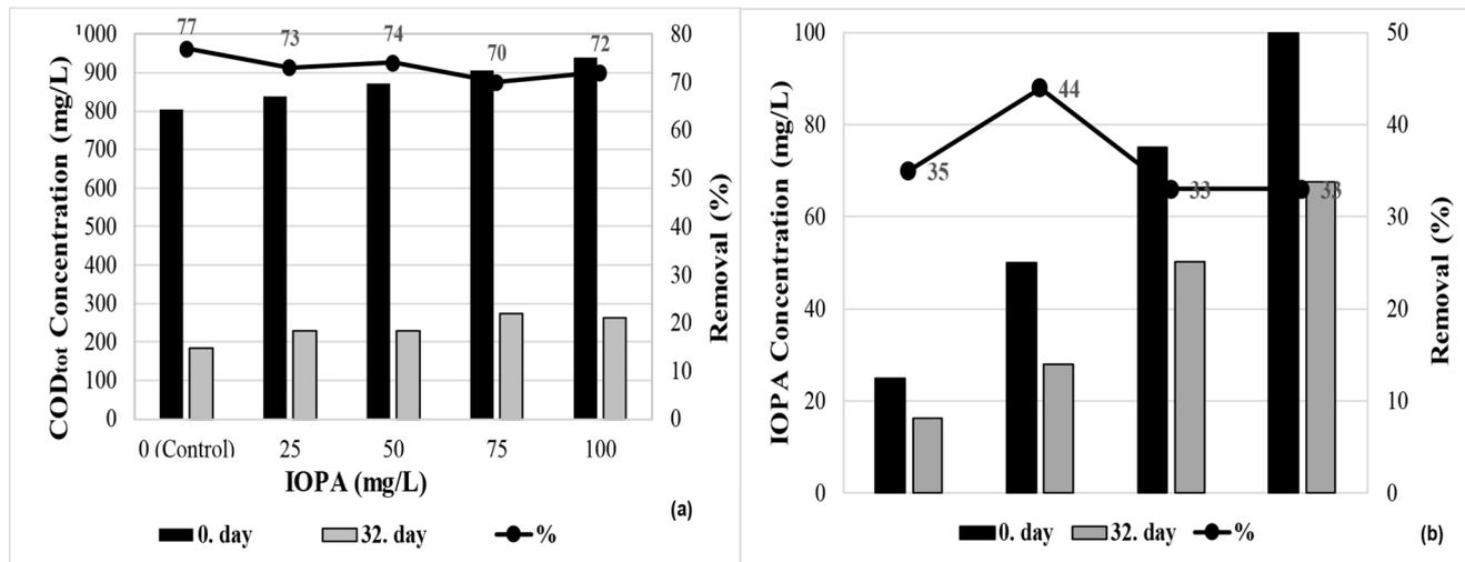
Fig. 1. Removals of (a) COD<sub>tot</sub> and (b) IOPA during anaerobic treatment of synthetic sewage (IOPA = 25–100 mg/L; T = 35°C; Incubation time = 32 d).
