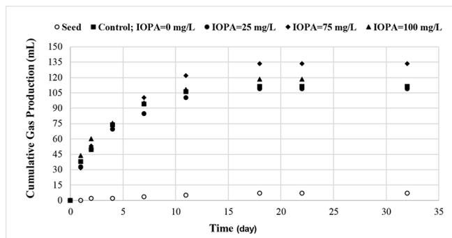
Fig. 2. Biogas productions at increasing IOPA in anaerobic bioreactors treating synthetic sewage (T = 35°C; Incubation time = 32 d; Initial COD<sub>tot</sub> = 800–950 mg/L).
